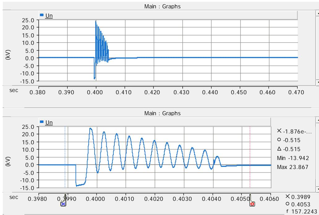
Figure 48. Reactor star point voltage on case 25.
