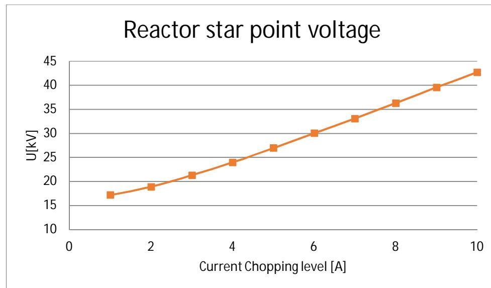
Figure 32. Peak values of shunt reactor star point voltage on cases 69-78 (Reactor 6 MVar, connection cable 15 m, main transformer 25 MVA)
