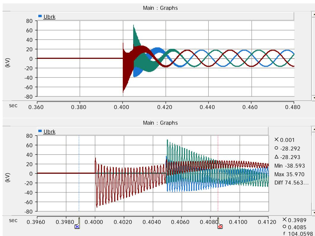
Figure 117. Breaker voltages before cable and reactor on case 135.
