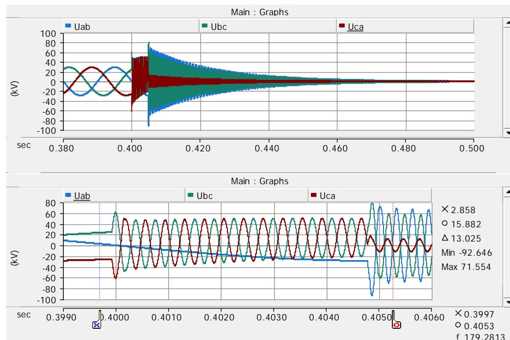
Figure 90. Reactor bus phase to phase voltages on case 100.
