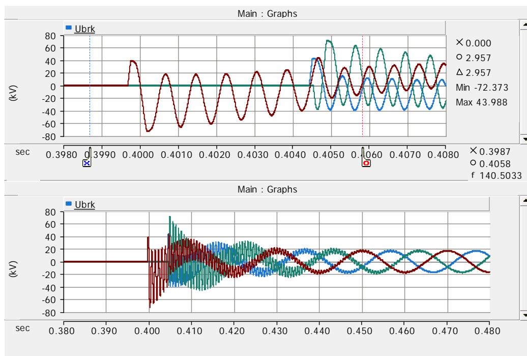
Figure 102. Breaker voltages before cable and reactor on case 114.
