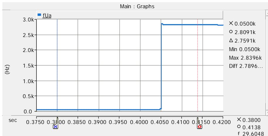
Figure 99. Ua phase Frequency on case 107.
