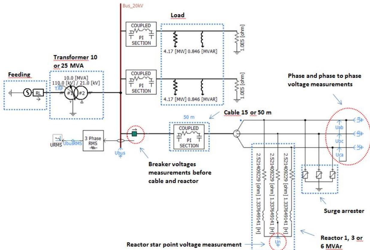
Figure 4. The simulation model.
