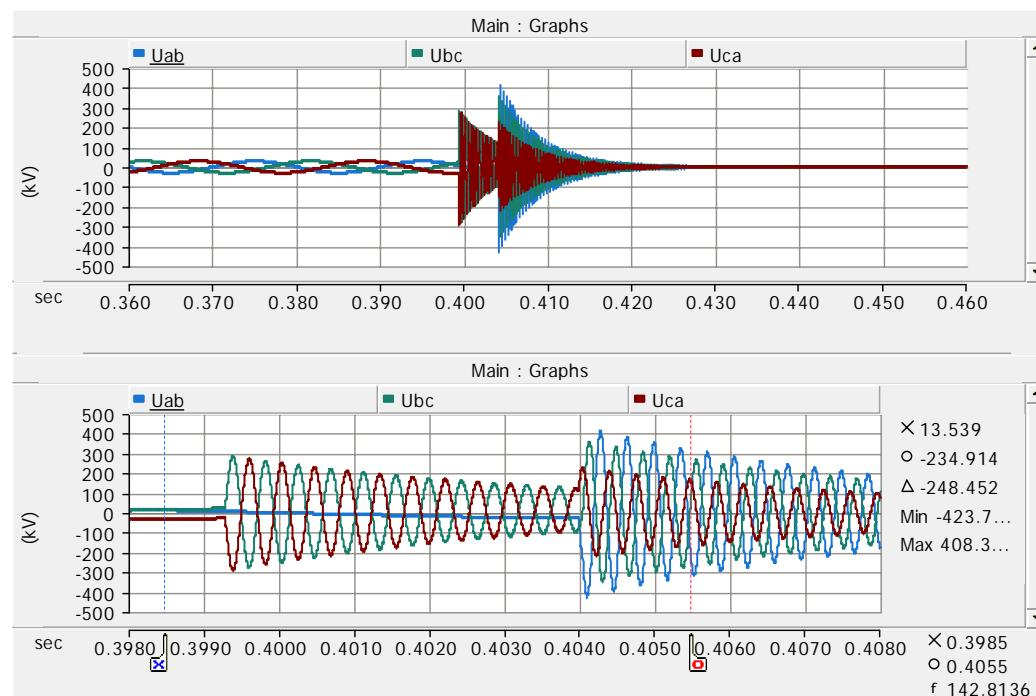
Figure 35. Reactor bus phase to phase voltages on case 10.
