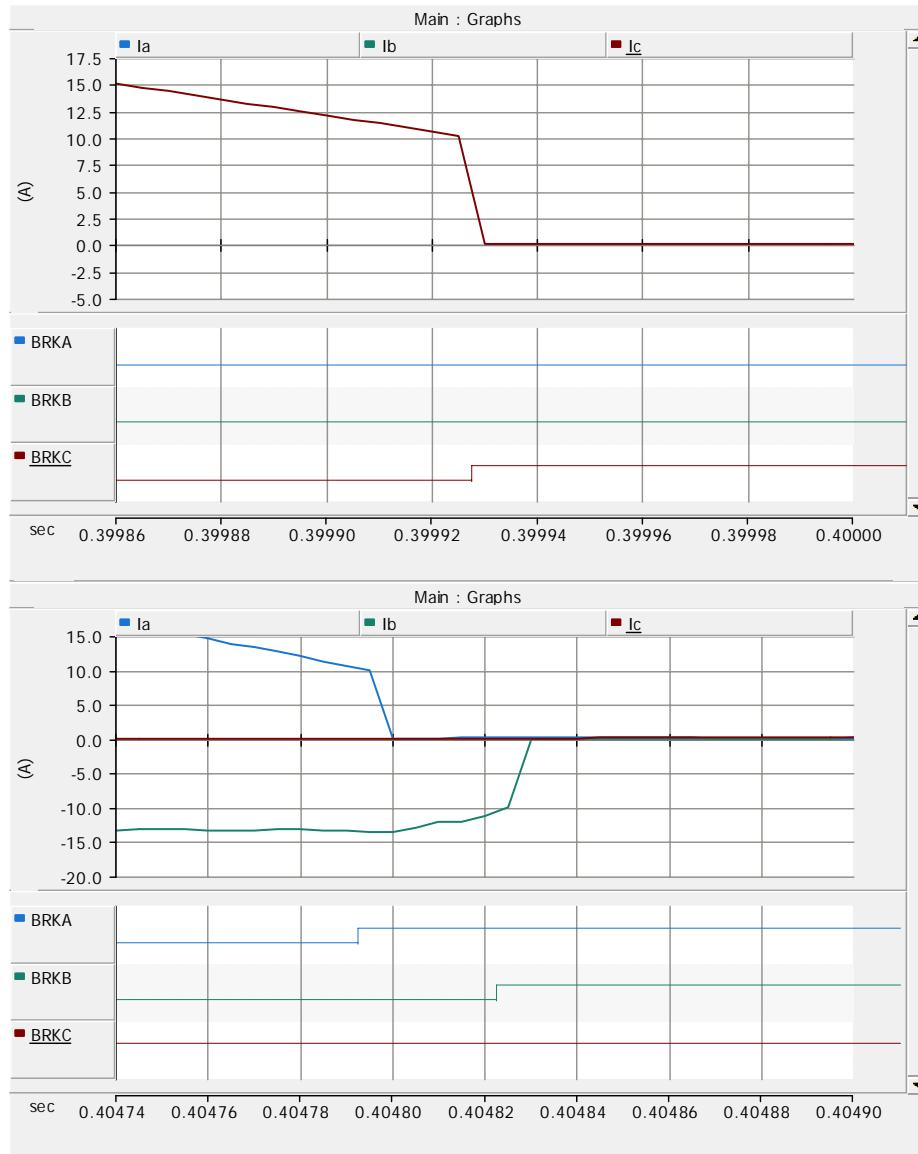
Figure 6. Single pole circuit breaker operation and current chopping in action.
