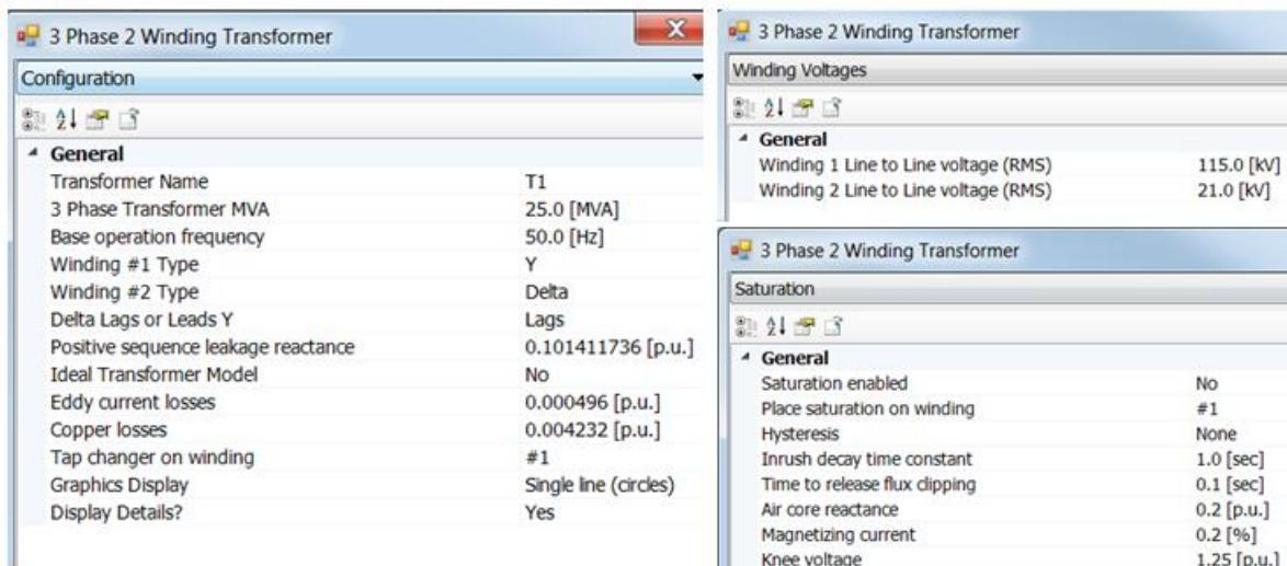
Figure 10. 25 MVA transformer parameters
