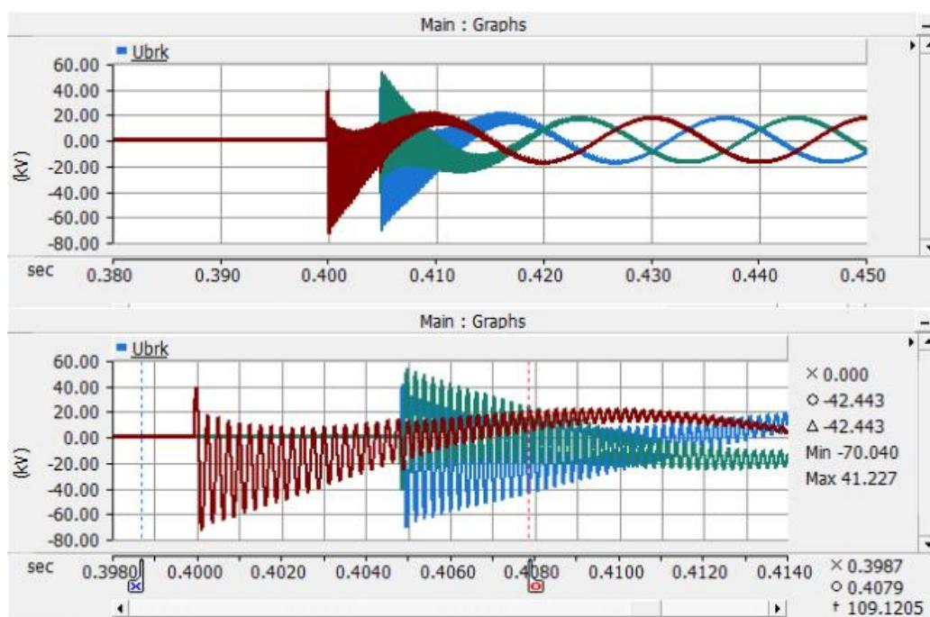
Figure 107. Breaker voltages before cable and reactor on case 121.
