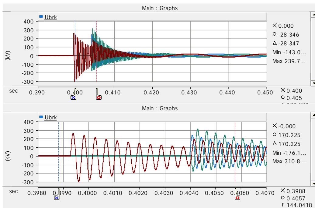
Figure 37. Breaker voltages before cable and reactor on case 10.
