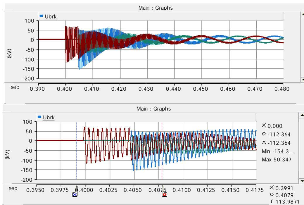
Figure 62. Breaker voltages before cable and reactor on case 54.
