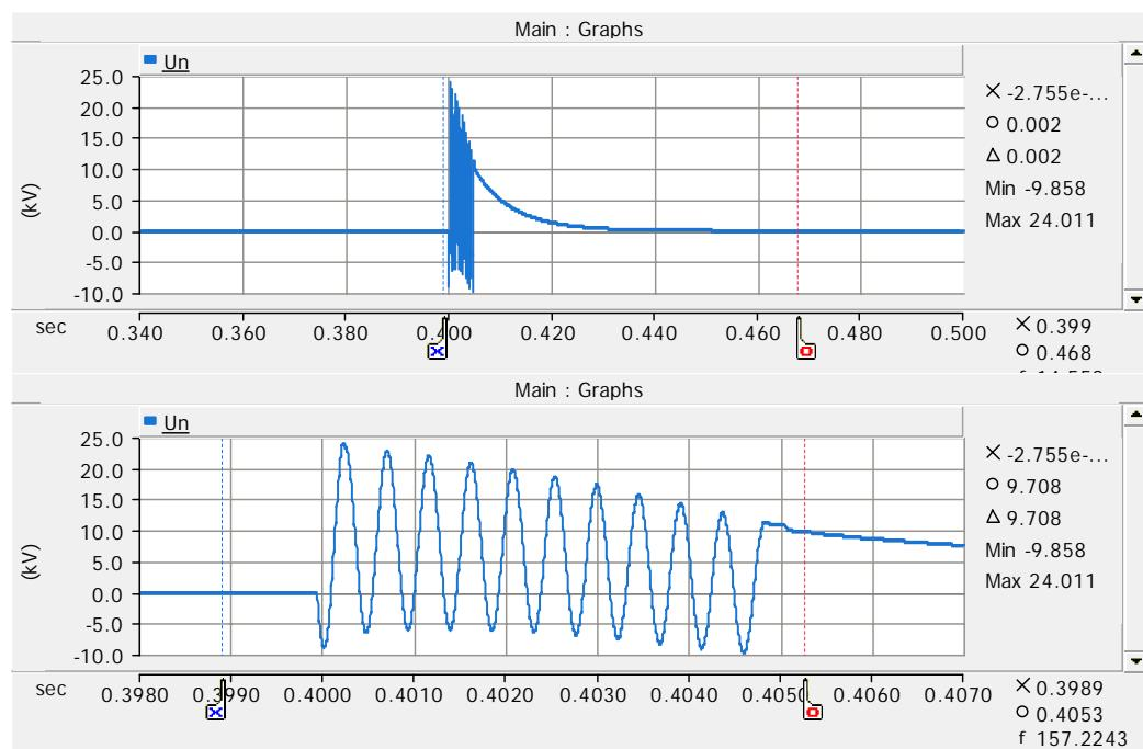
Figure 113. Reactor star point voltage on case 128.
