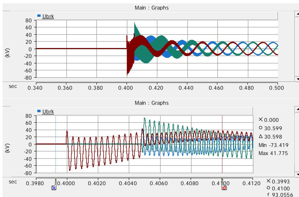
Figure 92. Breaker voltages before cable and reactor on case 100.
