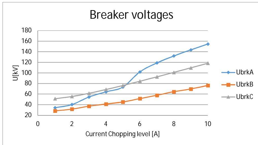
Figure 23. Peak values of breaker voltages on cases 45-54 (Reactor 3 MVar, connection cable 50 m, main transformer 25 MVA)
