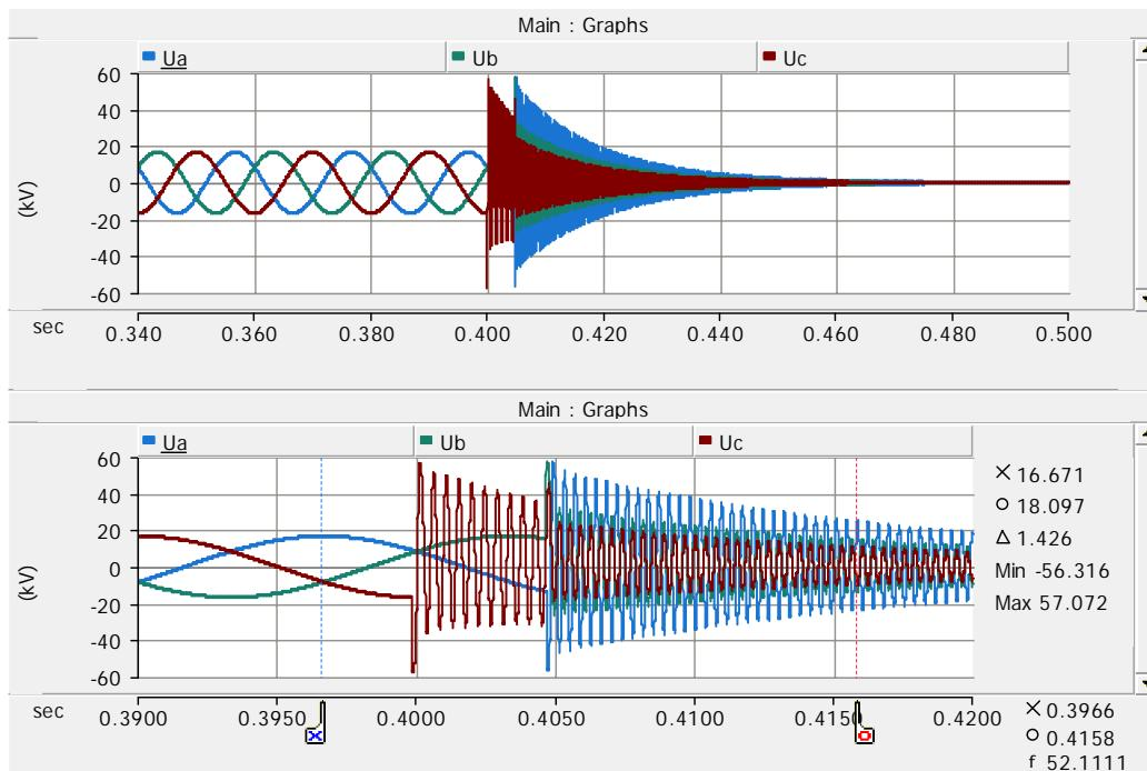
Figure 71. Reactor bus phase voltages on case 66.
