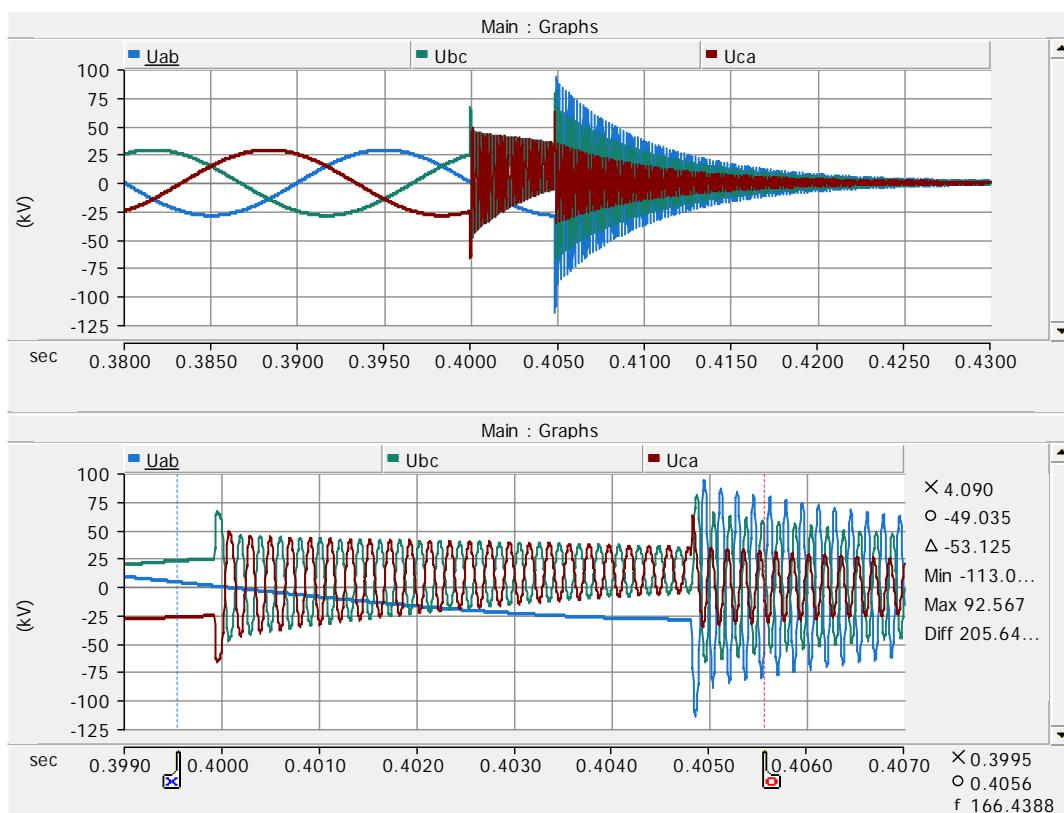
Figure 85. Reactor bus phase to phase voltages on case 93.
