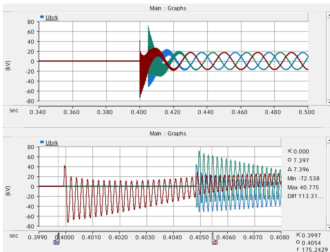
Figure 87. Breaker voltages before cable and reactor on case 93.
