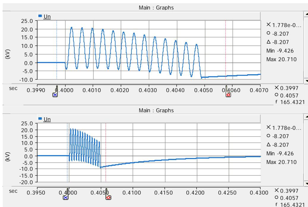
Figure 123. Reactor star point voltage on case 142.
