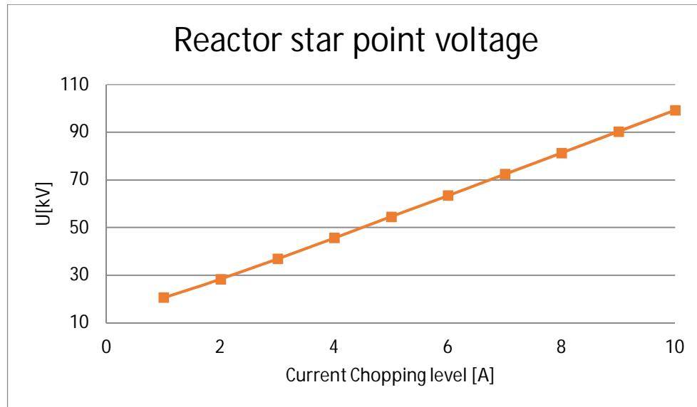
Figure 20. Peak values of shunt reactor star point voltage on cases 1-10 (Reactor 1 MVar, connection cable 15 m, main transformer 25 MVA)
