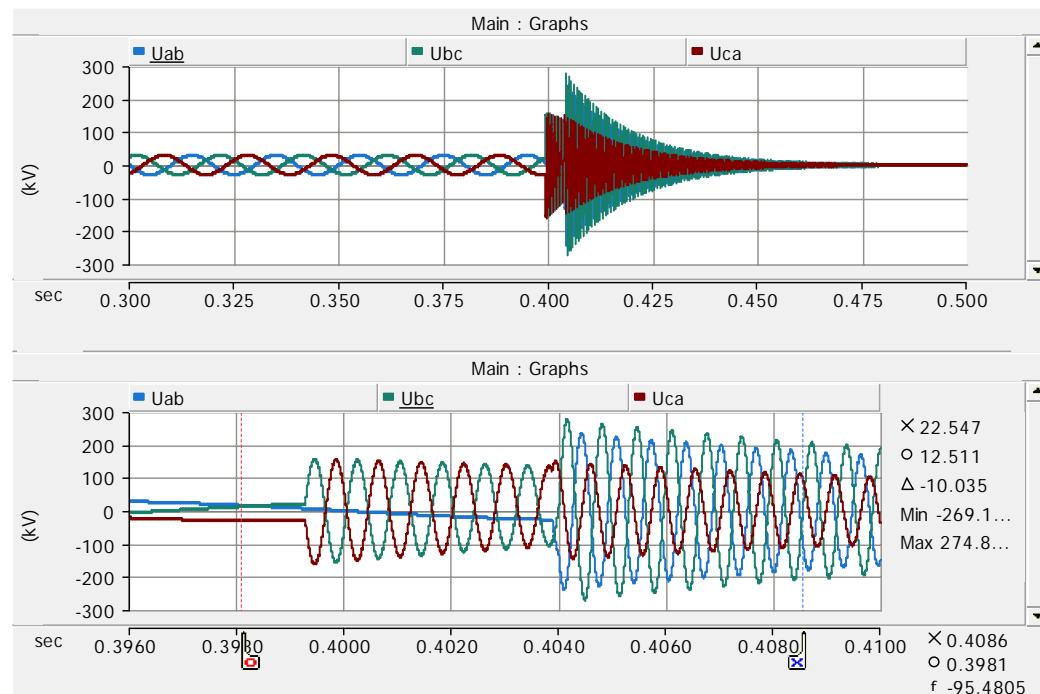
Figure 40. Reactor bus phase to phase voltages on case 20.
