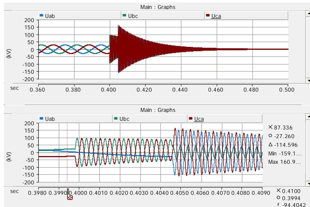
Figure 60. Reactor bus phase to phase voltages on case 54.
