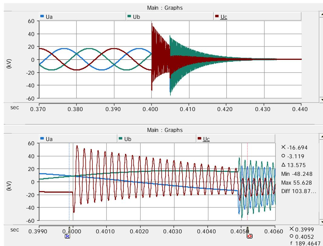
Figure 116. Reactor bus phase voltages on case 135.
