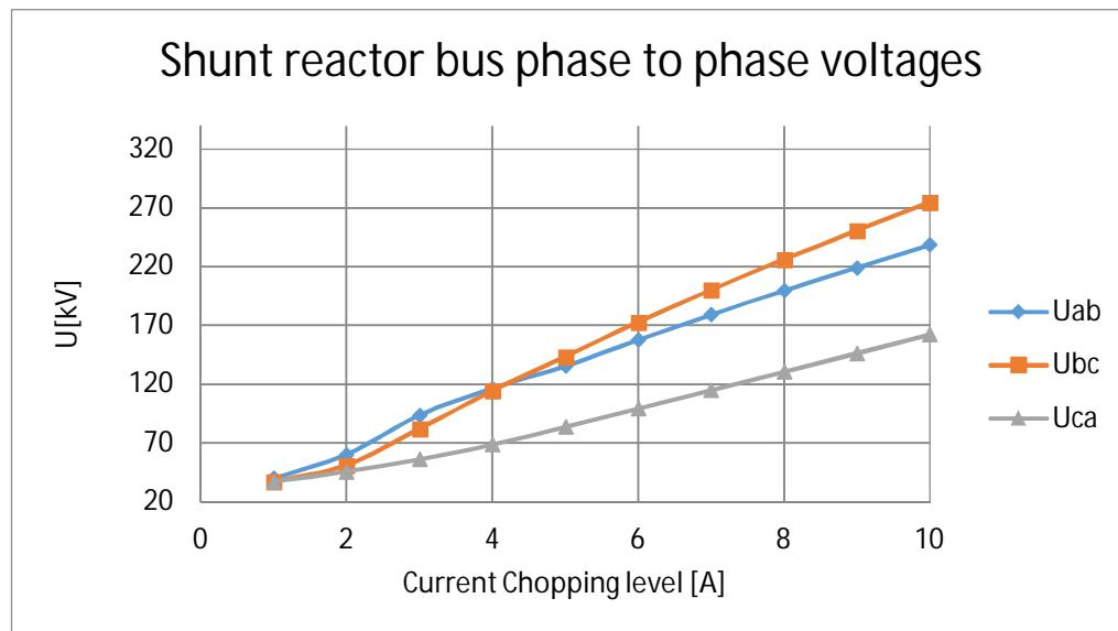
Figure 19. Peak values of shunt reactor bus phase voltages on cases 11-20 (Reactor 1 MVar, connection cable 50 m, main transformer 25 MVA)
