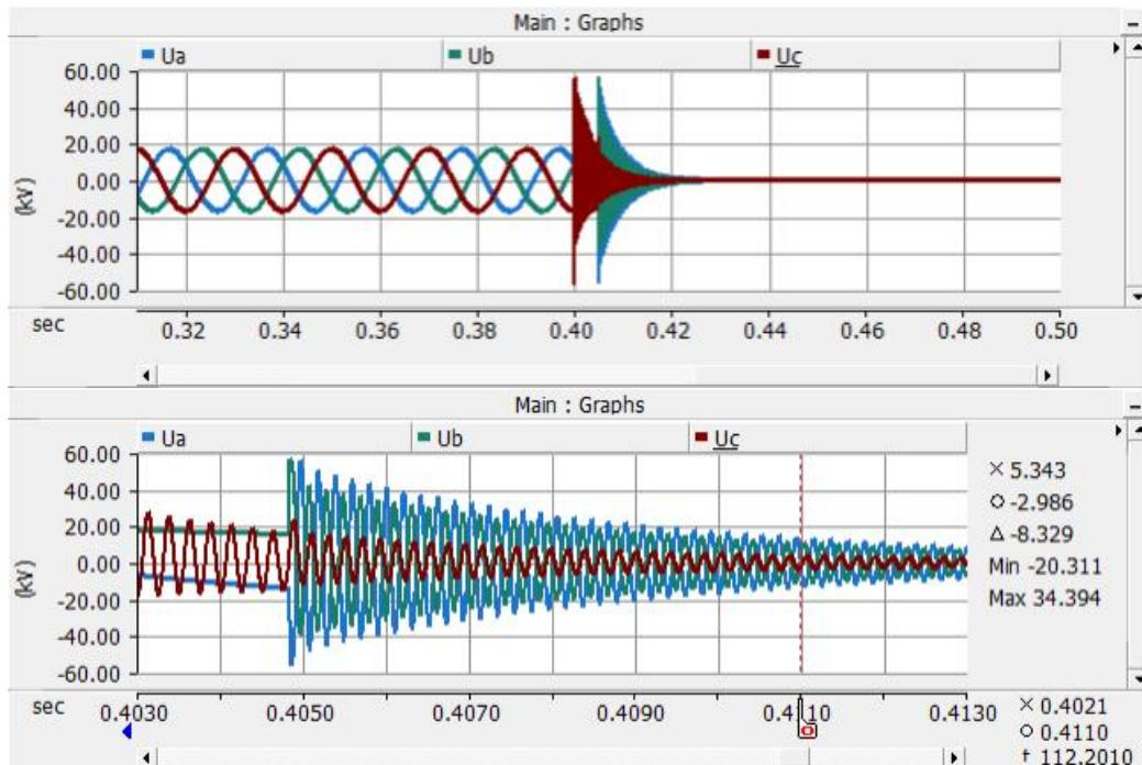
Figure 106. Reactor bus phase voltages on case 121.
