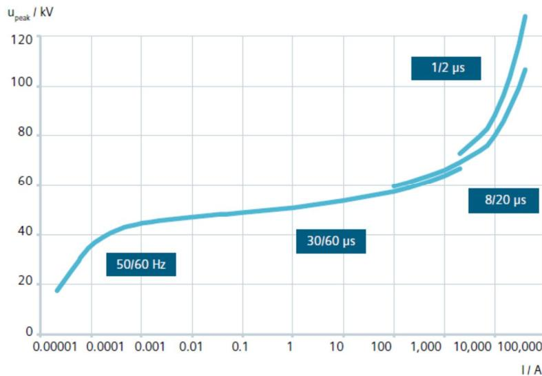
Figure 13. Example of voltage-current characteristic of a 30 kV surge arrester.
