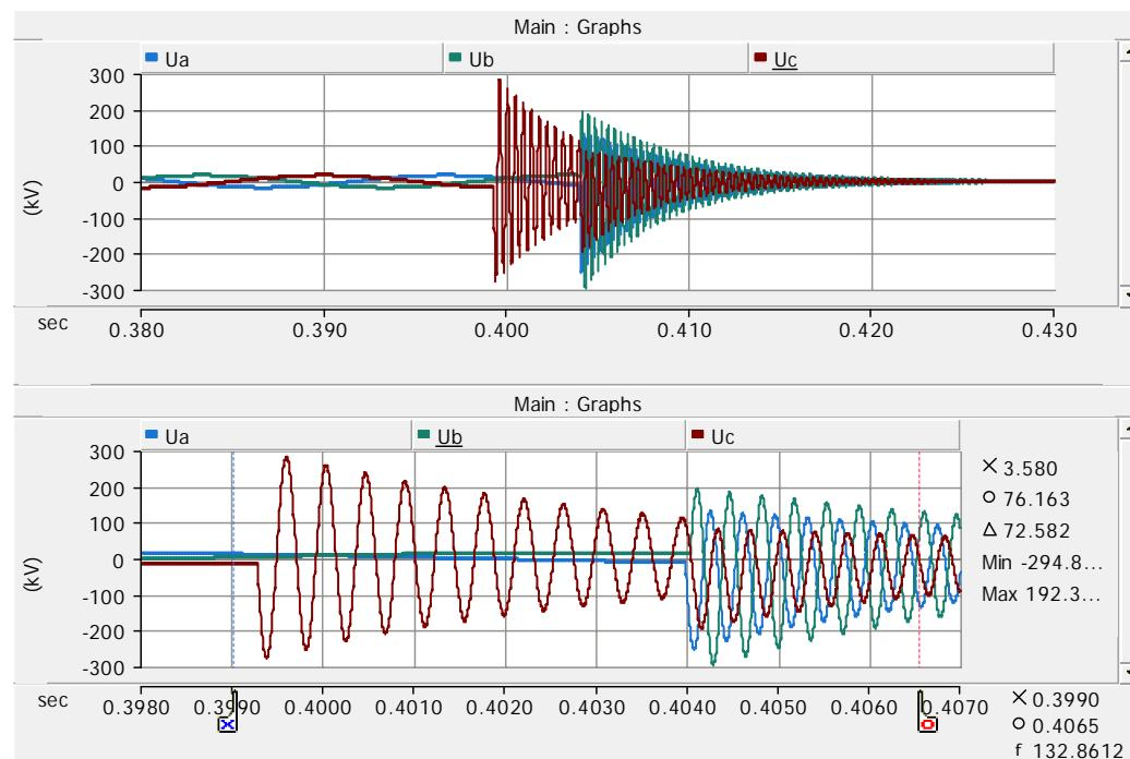
Figure 36. Reactor bus phase voltages on case 10.
