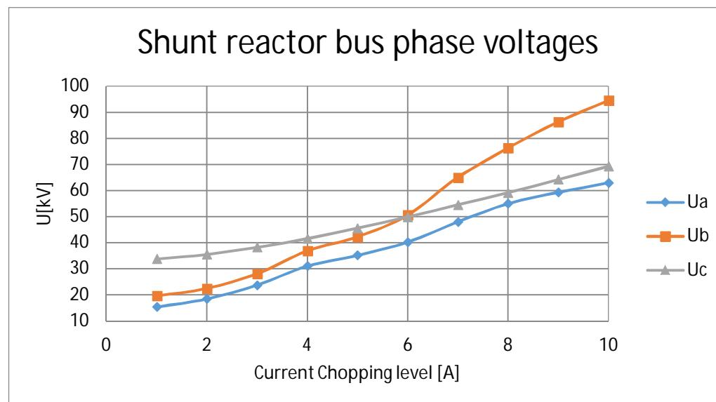
Figure 31. Peak values of shunt reactor bus phase voltages on cases 79-88 (Reactor 6 MVar, connection cable 50 m, main transformer 25 MVA)
