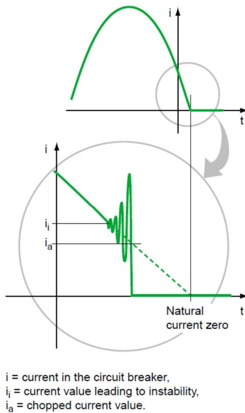
Figure 1. The high frequency oscillation phenomena leading to current chopping [1].
