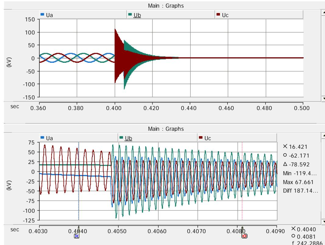
Figure 76. Reactor bus phase voltages on case 78.
