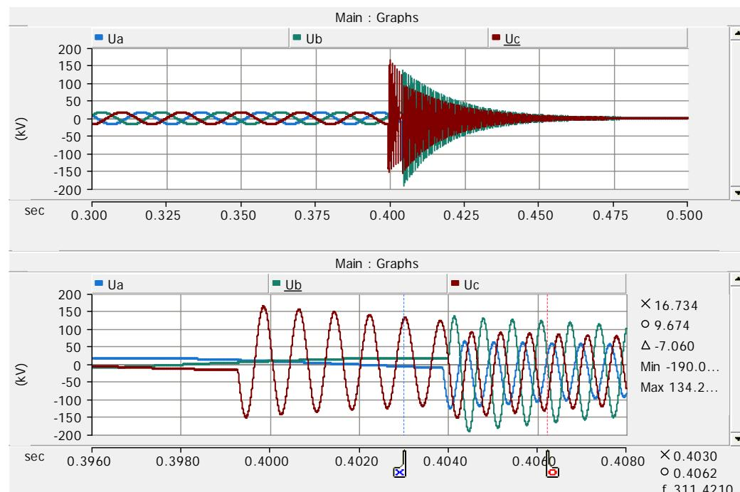
Figure 41. Reactor bus phase voltages on case 20.
