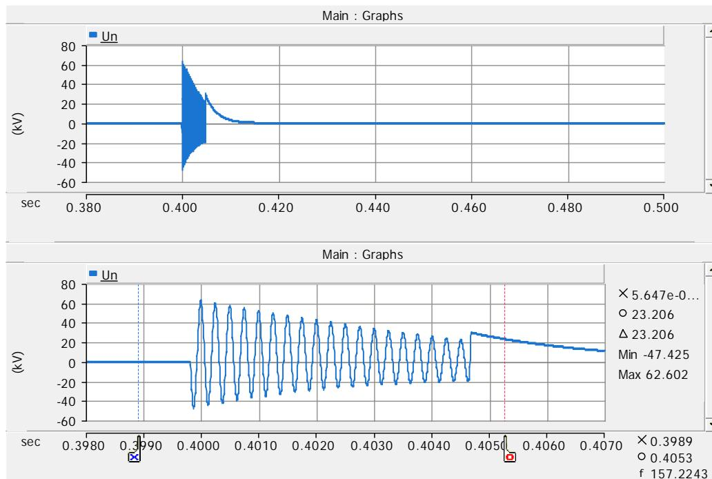
Figure 58. Reactor star point voltage on case 44.
