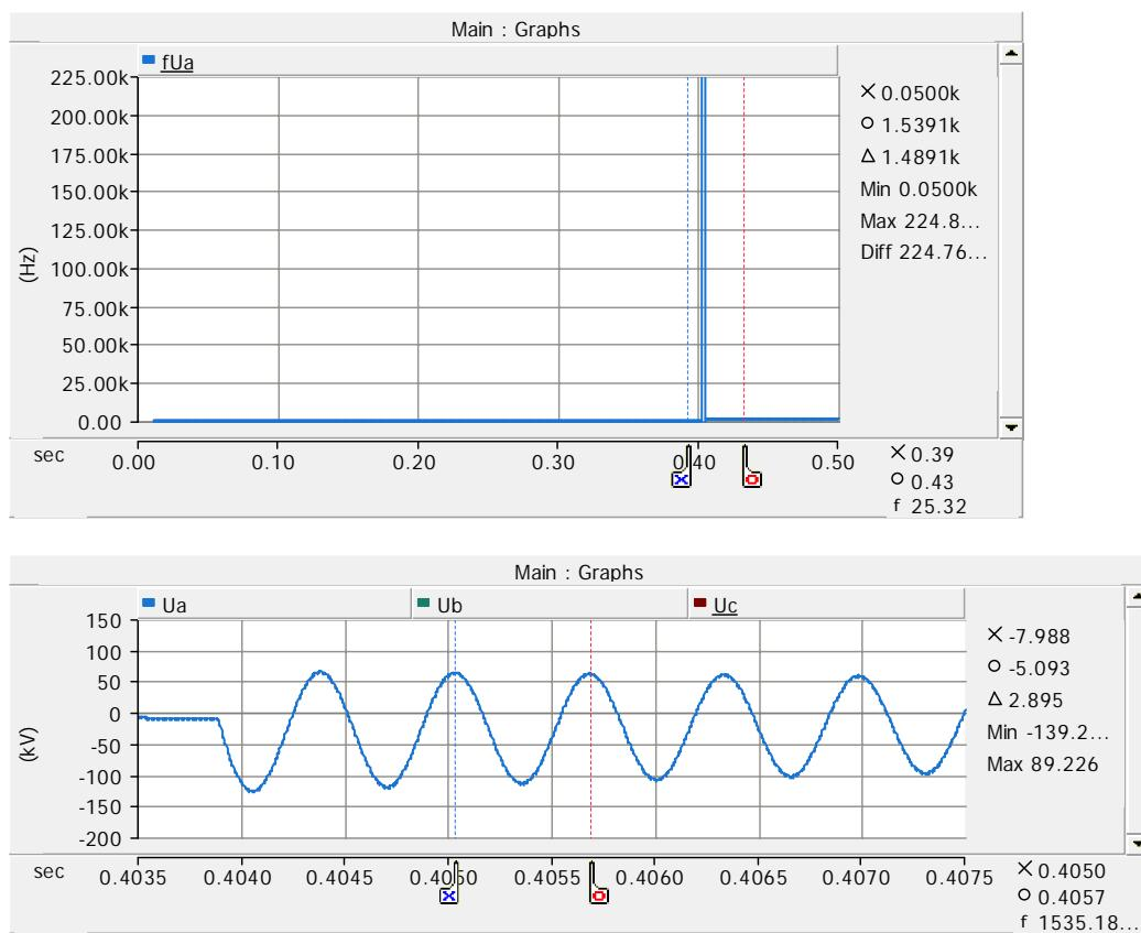
Figure 44.  $U_a$  phase Frequency on case 20.
