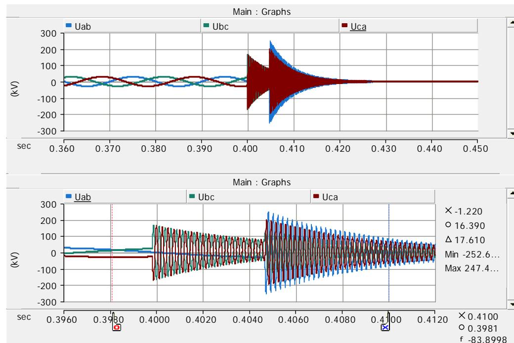
Figure 55. Reactor bus phase to phase voltages on case 44.
