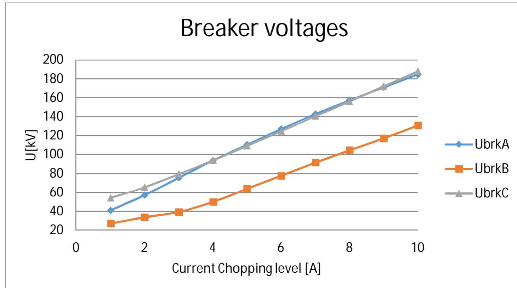
Figure 22. Peak values of breaker voltages on cases 35-44 (Reactor 3 MVar, connection cable 15 m, main transformer 25 MVA)
