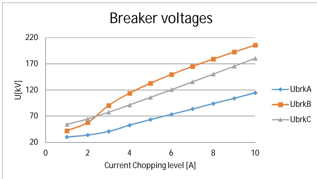
Figure 17. Peak values of breaker voltages on cases 11-20 (Reactor 1 MVar, connection cable 50 m, main transformer 25 MVA)
