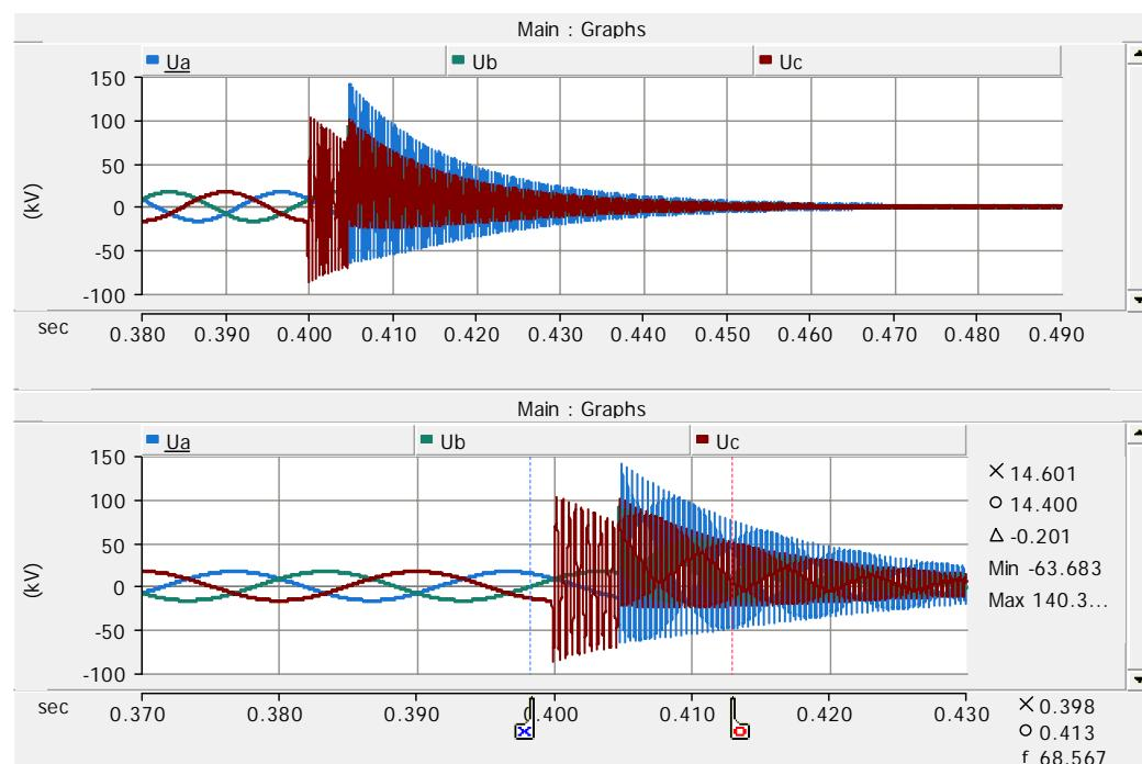
Figure 61. Reactor bus phase voltages on case 54.
