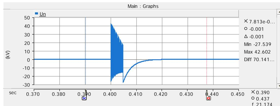
Figure 78. Reactor star point voltage on case 78.
