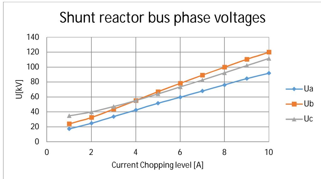
Figure 30. Peak values of shunt reactor bus phase voltages on cases 69-78 (Reactor 6 MVar, connection cable 15 m, main transformer 25 MVA)
