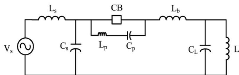
Figure 2. Single-phase equivalent circuit for shunt reactor switching transient analysis [2].
