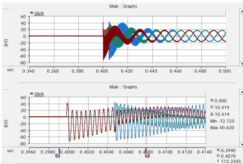
Figure 72. Breaker voltages before cable and reactor on case 66.
