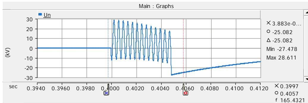
Figure 83. Reactor star point voltage on case 88.
