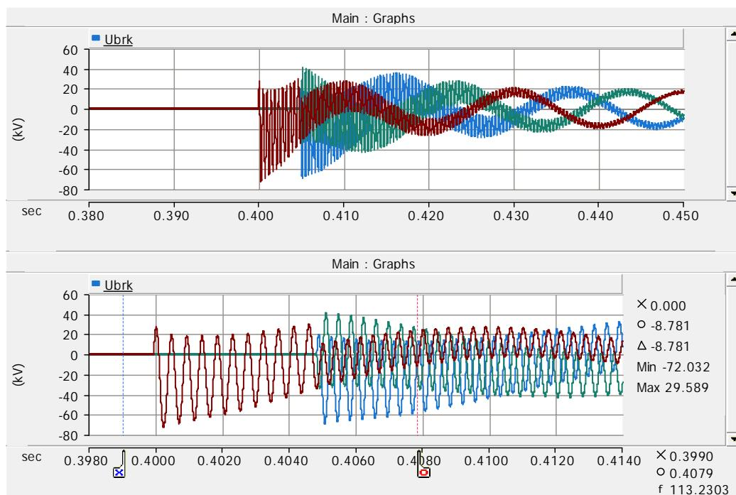
Figure 112. Breaker voltages before cable and reactor on case 128.
