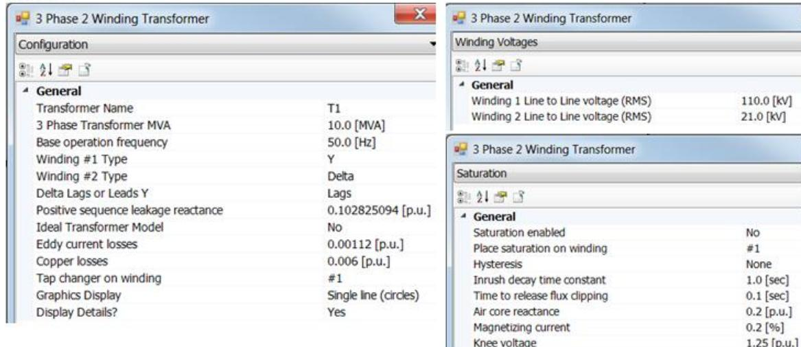
Figure 11. 10 MVA transformer parameters
