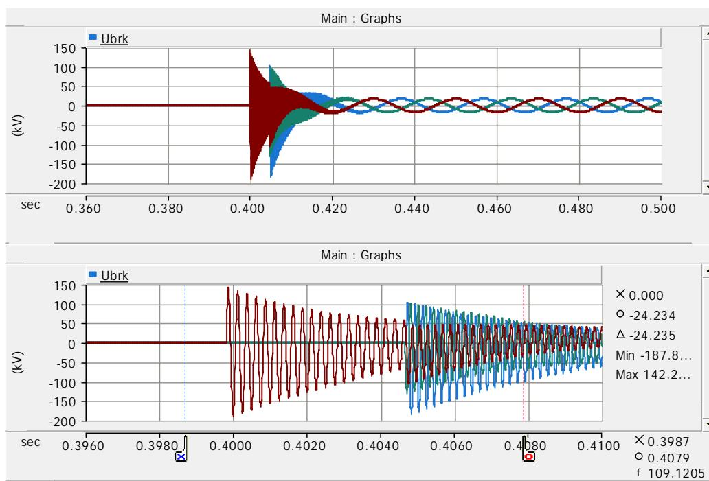
Figure 57. Breaker voltages before cable and reactor on case 44.
