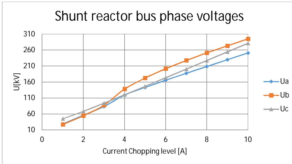
Figure 18. Peak values of shunt reactor bus phase voltages on cases 1-10 (Reactor 1 MVar, connection cable 15 m, main transformer 25 MVA)
