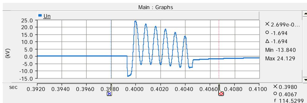
Figure 53. Reactor star point voltage on case 32.
