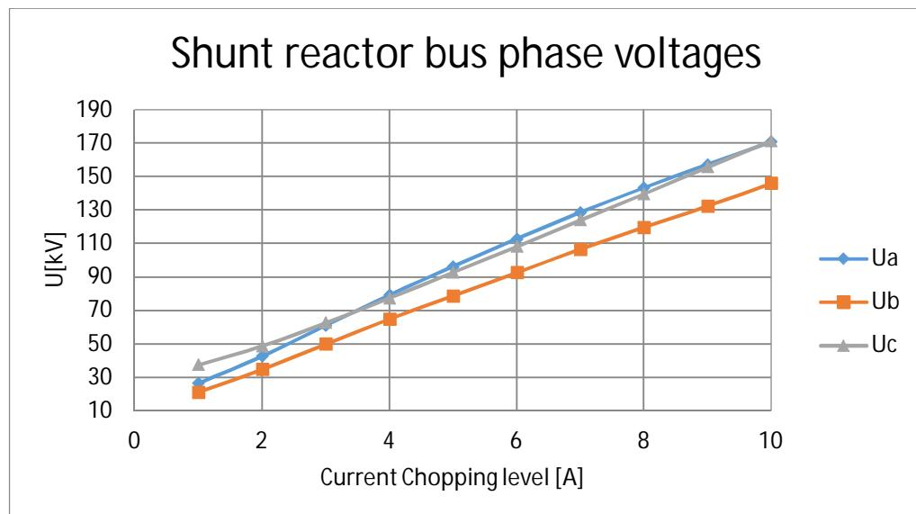
Figure 24. Peak values of shunt reactor bus phase voltages on cases 35-44 (Reactor 3 MVar, connection cable 15 m, main transformer 25 MVA)
