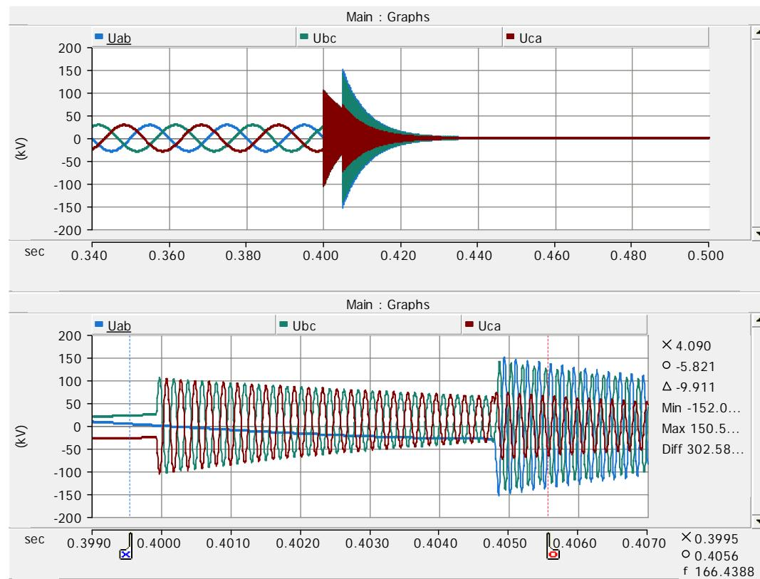
Figure 75. Reactor bus phase to phase voltages on case 78.
