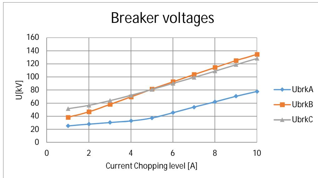
Figure 28. Peak values of breaker voltages on cases 69-78 (Reactor 6 MVAr, connection cable 15 m, main transformer 25 MVA)
