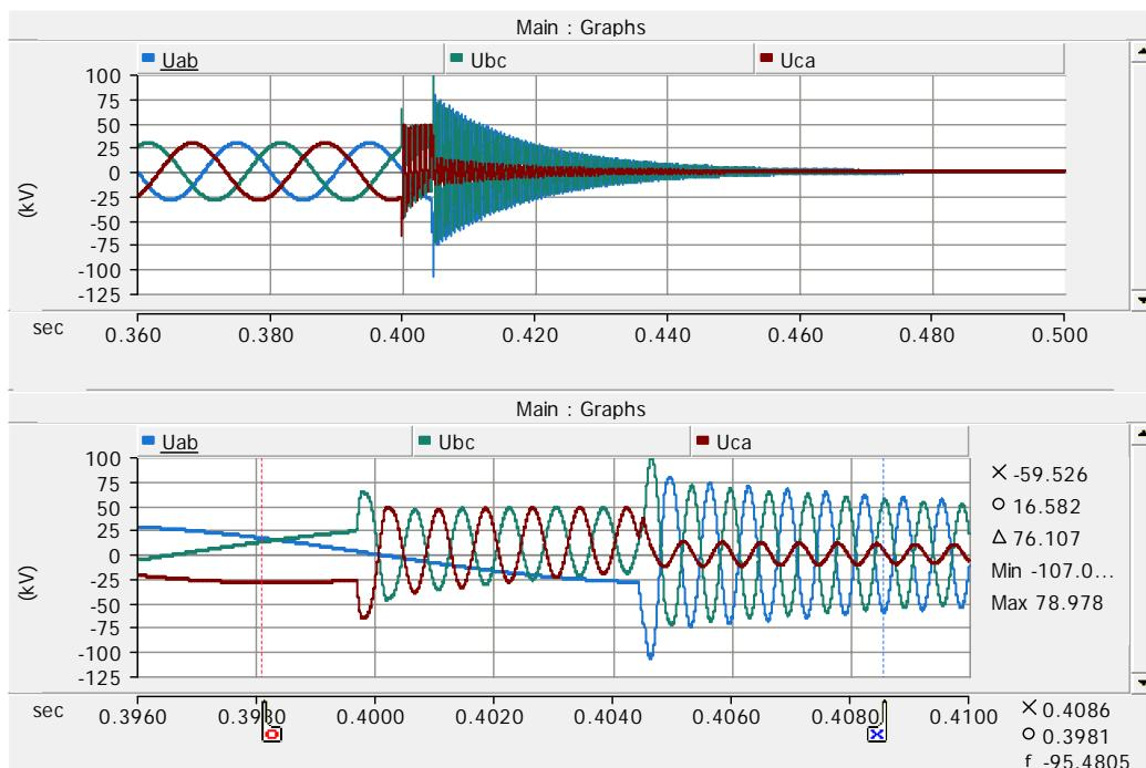
Figure 100. Reactor bus phase to phase voltages on case 114.
