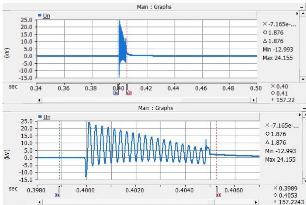
Figure 108. Reactor star point voltage on case 121.
