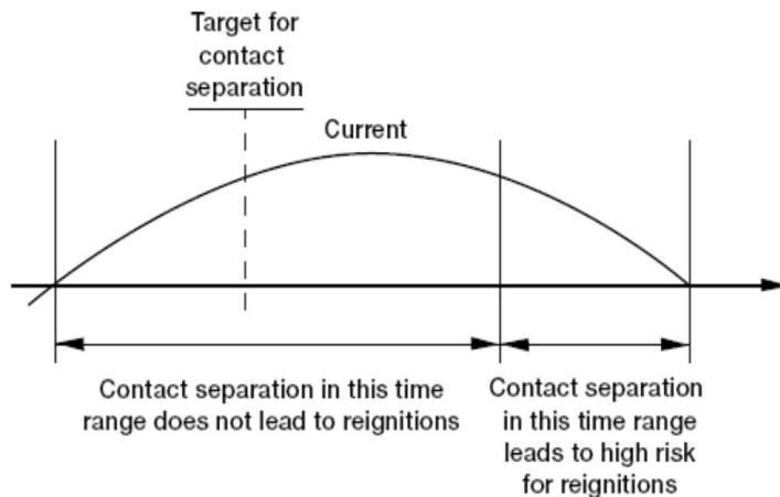
Figure 3. Target for contact separation to eliminate re-ignition [10].
