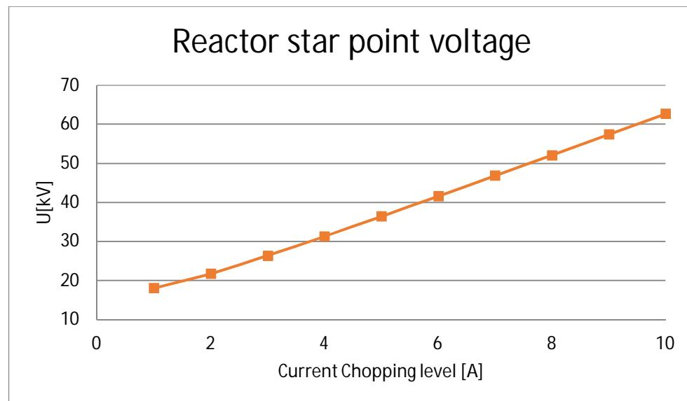
Figure 26. Peak values of shunt reactor star point voltages on cases 35-44 (Reactor 3 MVar, connection cable 15 m, main transformer 25 MVA)
