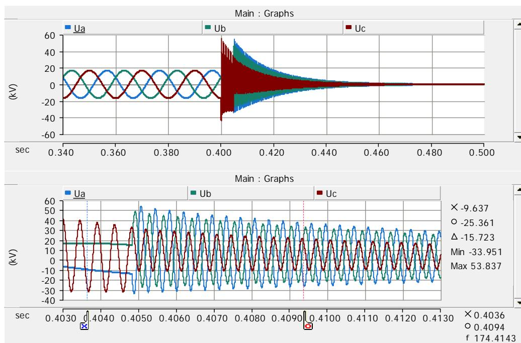
Figure 111. Reactor bus phase voltages on case 128.
