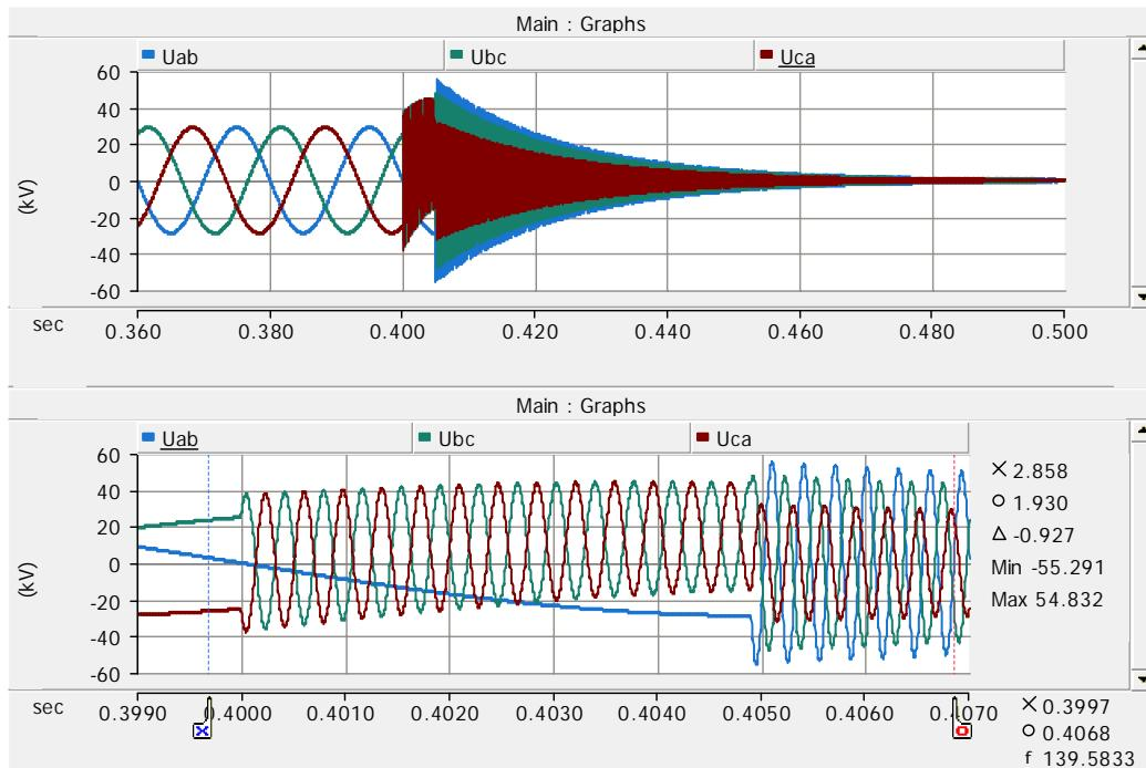
Figure 120. Reactor bus phase to phase voltages on case 142.
