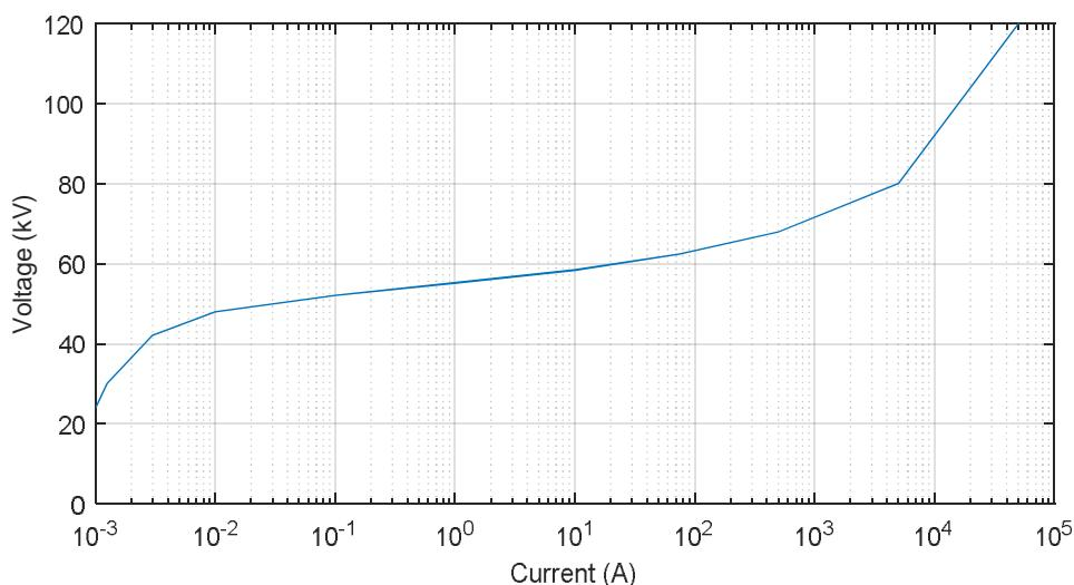
Figure 15. Voltage-current characteristic of the modelled surge arrester.
