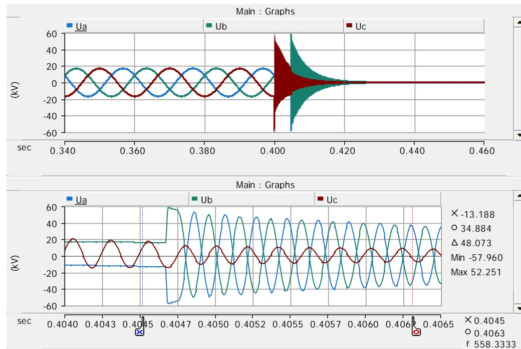
Figure 66. Reactor bus phase voltages on case 59.
