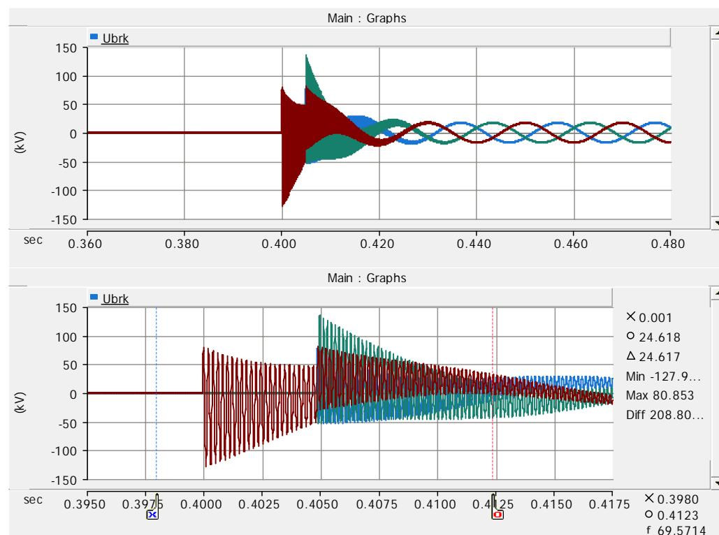
Figure 77. Breaker voltages before cable and reactor on case 78.
