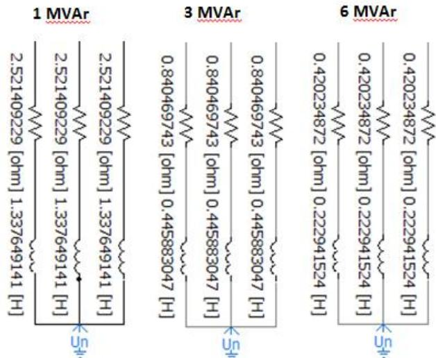
Figure 7. Simulation models for all three reactors
