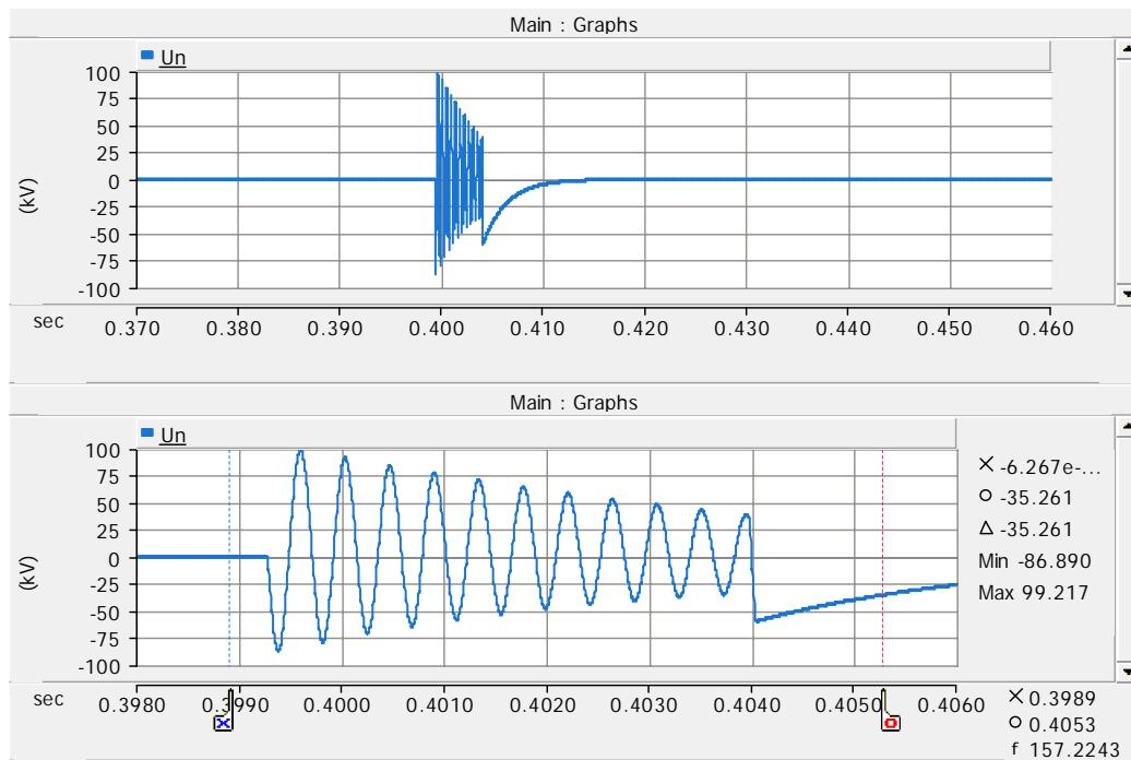
Figure 38. Reactor star point voltage on case 10.
