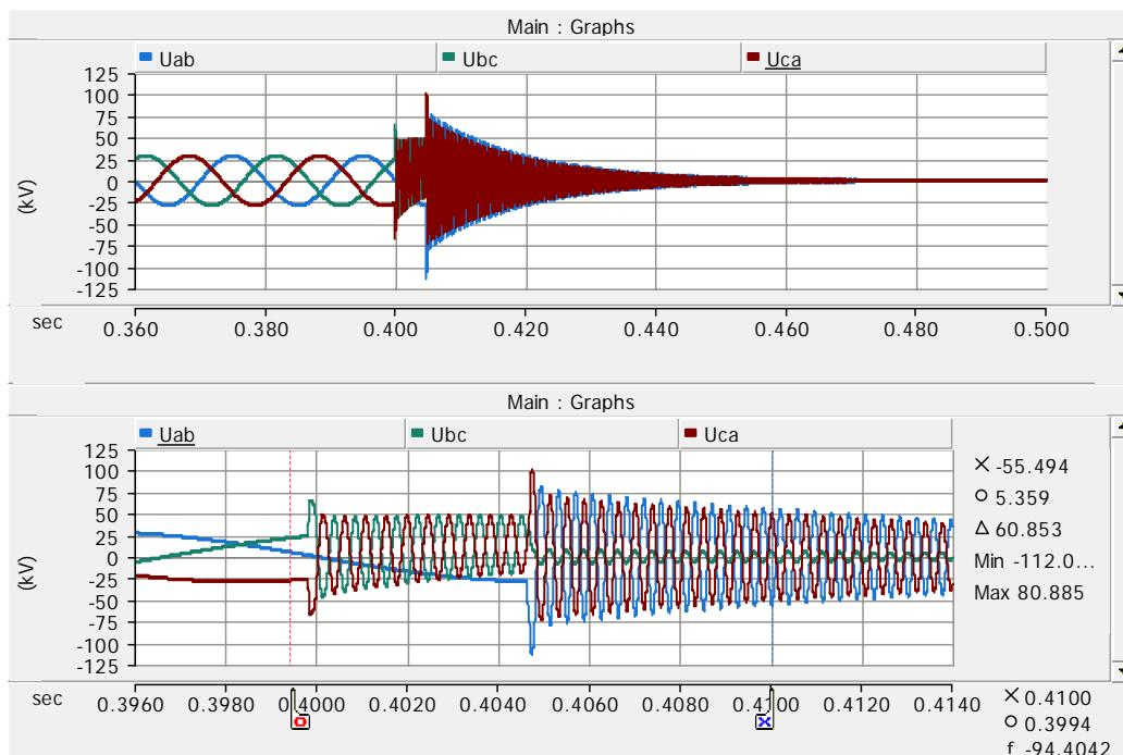
Figure 70. Reactor bus phase to phase voltages on case 66.
