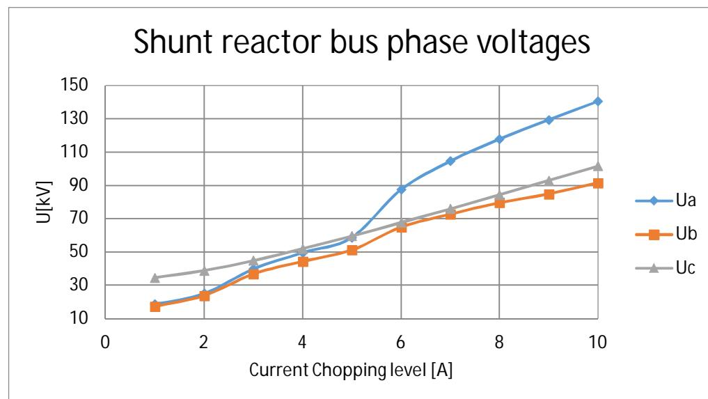
Figure 25. Peak values of shunt reactor bus phase voltages on cases 45-54 (Reactor 3 MVar, connection cable 50 m, main transformer 25 MVA)
