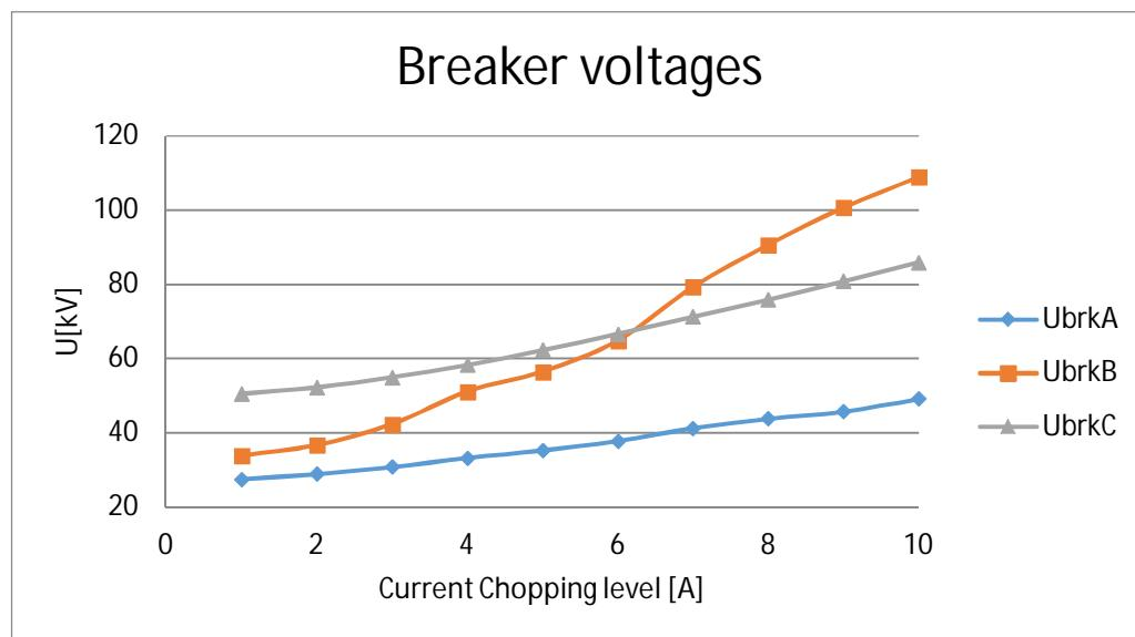
Figure 29. Peak values of breaker voltages on cases 79-88 (Reactor 6 MVar, connection cable 50 m, main transformer 25 MVA)
