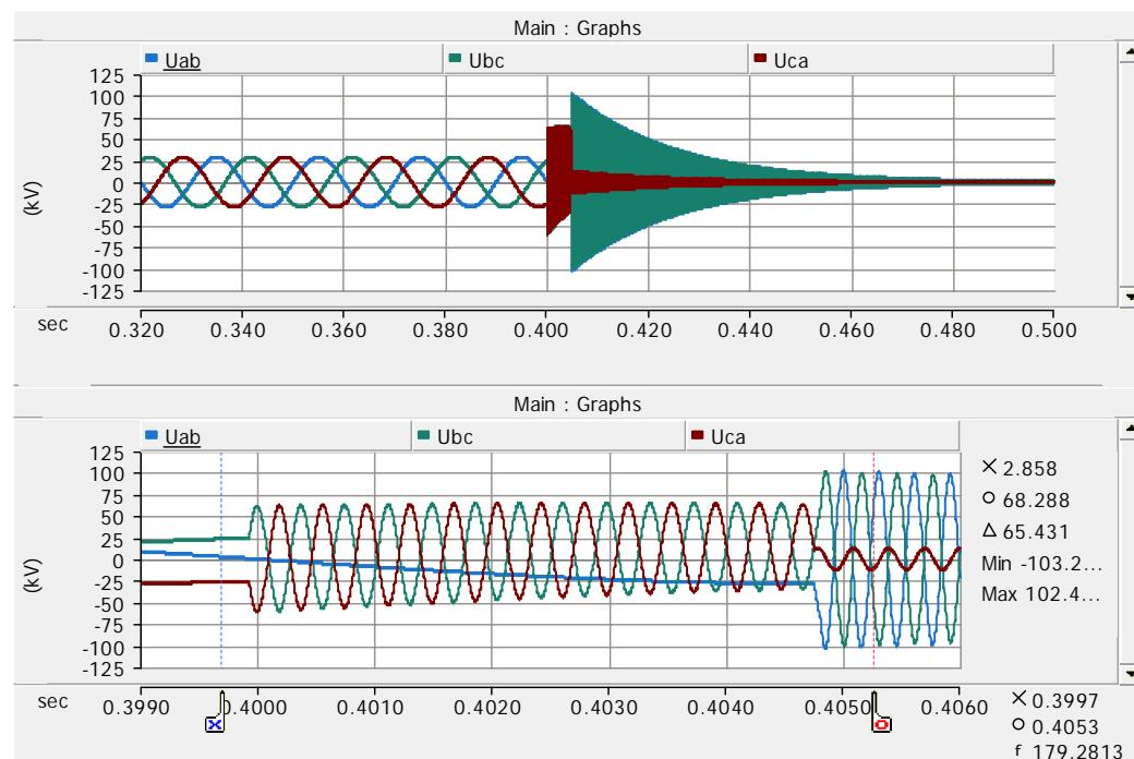
Figure 80. Reactor bus phase to phase voltages on case 88.
