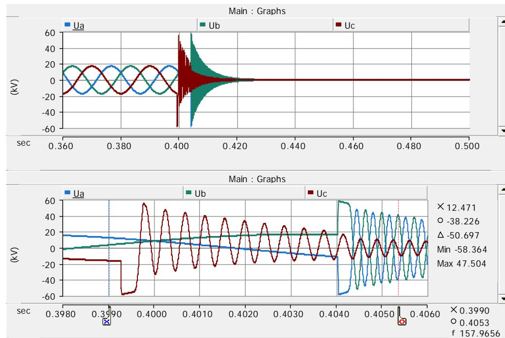
Figure 46. Reactor bus phase voltages on case 25.
