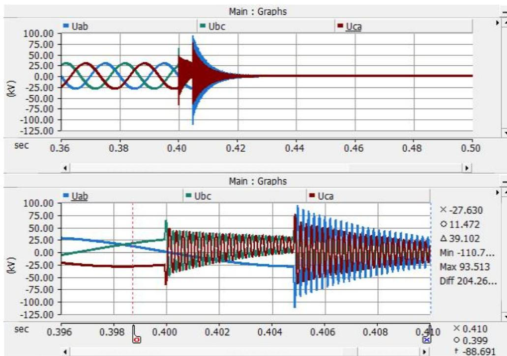
Figure 105. Reactor bus phase to phase voltages on case 121.
