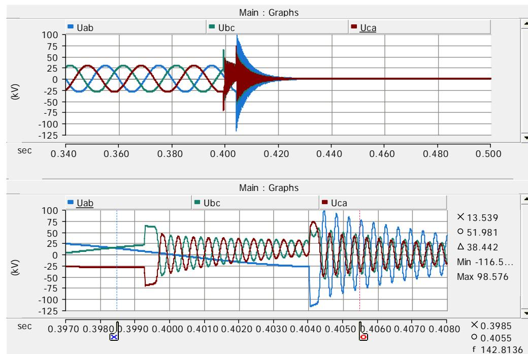
Figure 45. Reactor bus phase to phase voltages on case 25.
