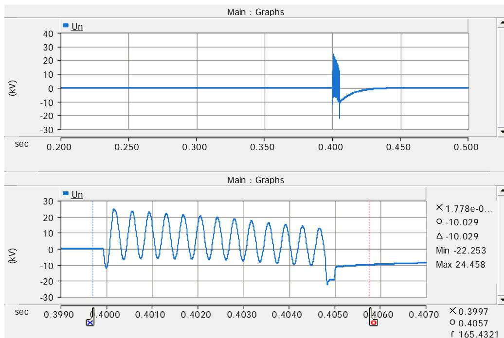
Figure 93. Reactor star point voltage on case 100.
