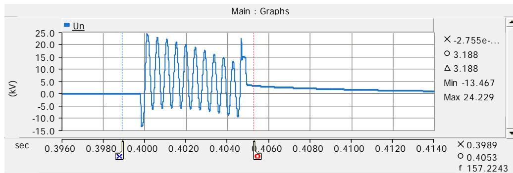
Figure 73. Reactor star point voltage on case 66.
