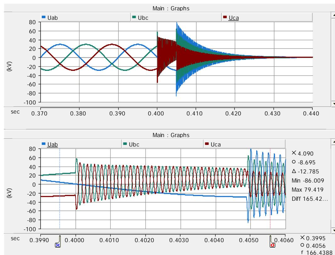
Figure 115. Reactor bus phase to phase voltages on case 135.
