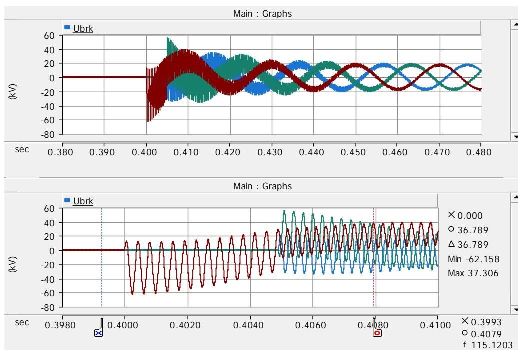
Figure 122. Breaker voltages before cable and reactor on case 142.
