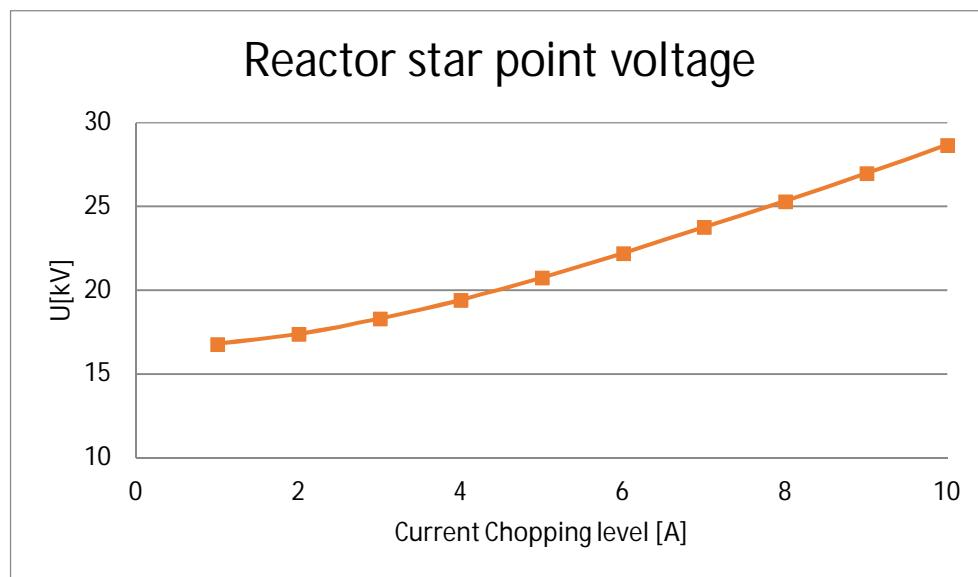
Figure 33. Peak values of shunt reactor star point voltage on cases 79-88 (Reactor 6 MVar, connection cable 50 m, main transformer 25 MVA)
