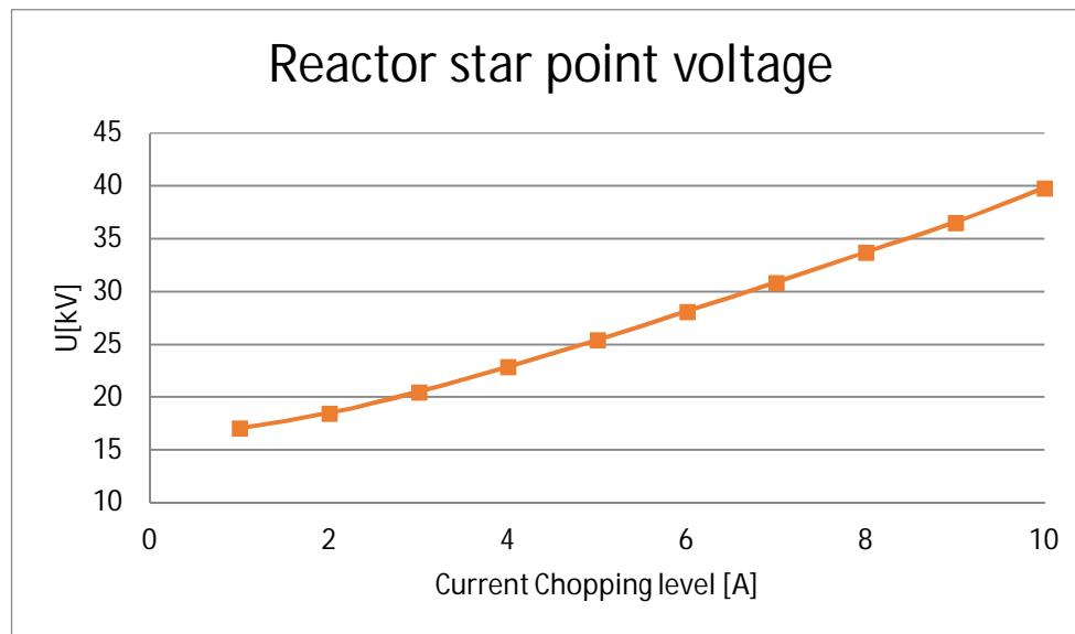
Figure 27. Peak values of shunt reactor star point voltage on cases 45-54 (Reactor 3 MVar, connection cable 50 m, main transformer 25 MVA)
