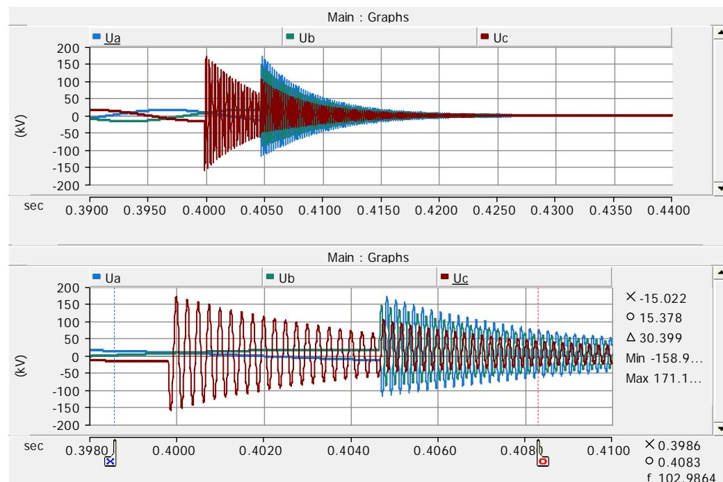
Figure 56. Reactor bus phase voltages on case 44.
