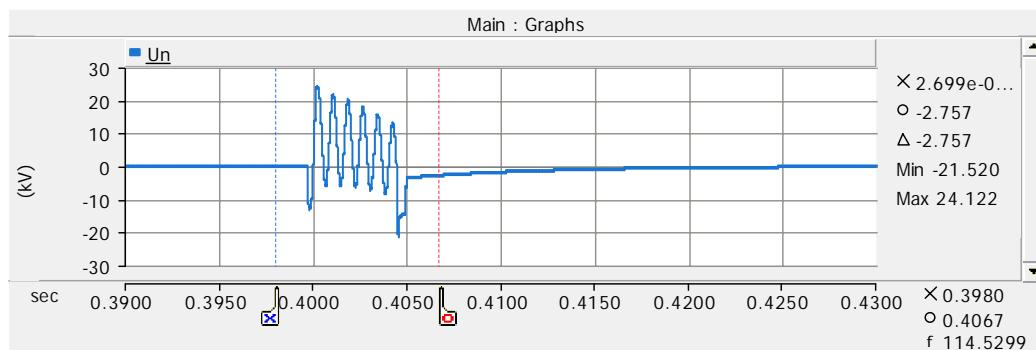
Figure 103. Reactor star point voltage on case 114.
