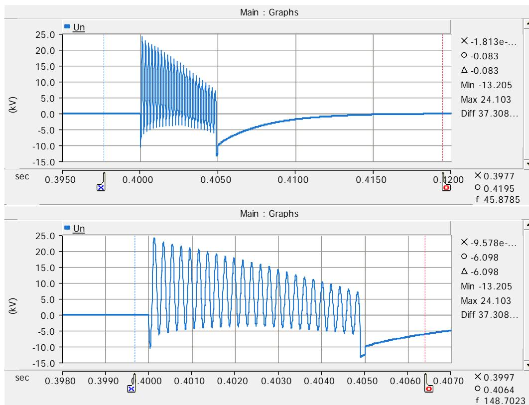
Figure 118. Reactor star point voltage on case 135.
