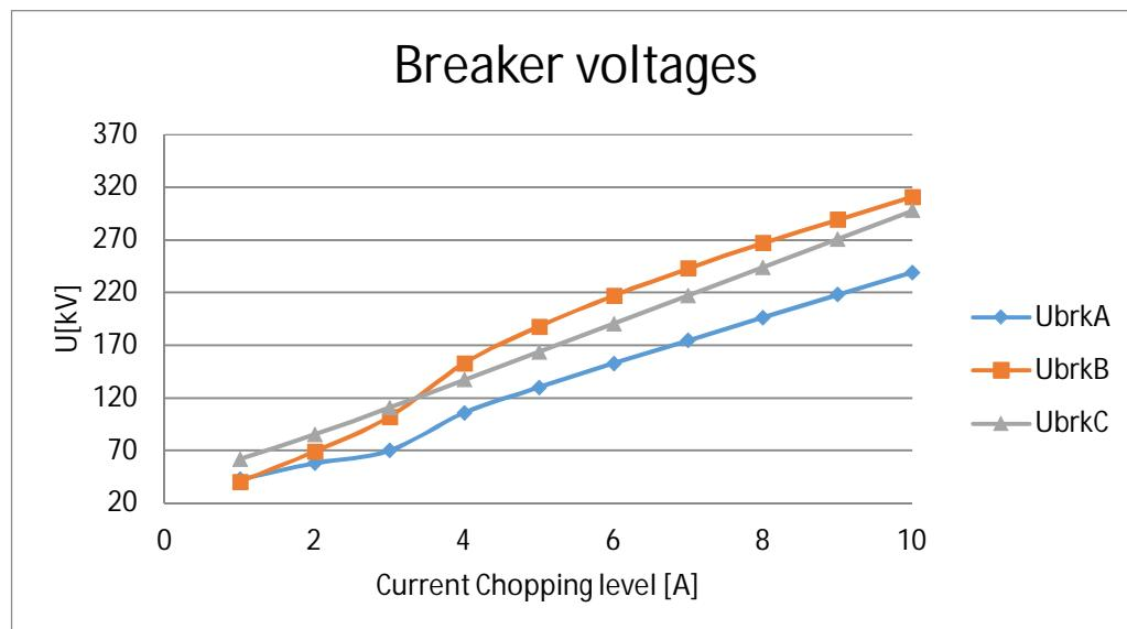
Figure 16. Peak values of breaker voltages on cases 1-10 (Reactor 1 MVAr, connection cable 15 m, main transformer 25 MVA)
