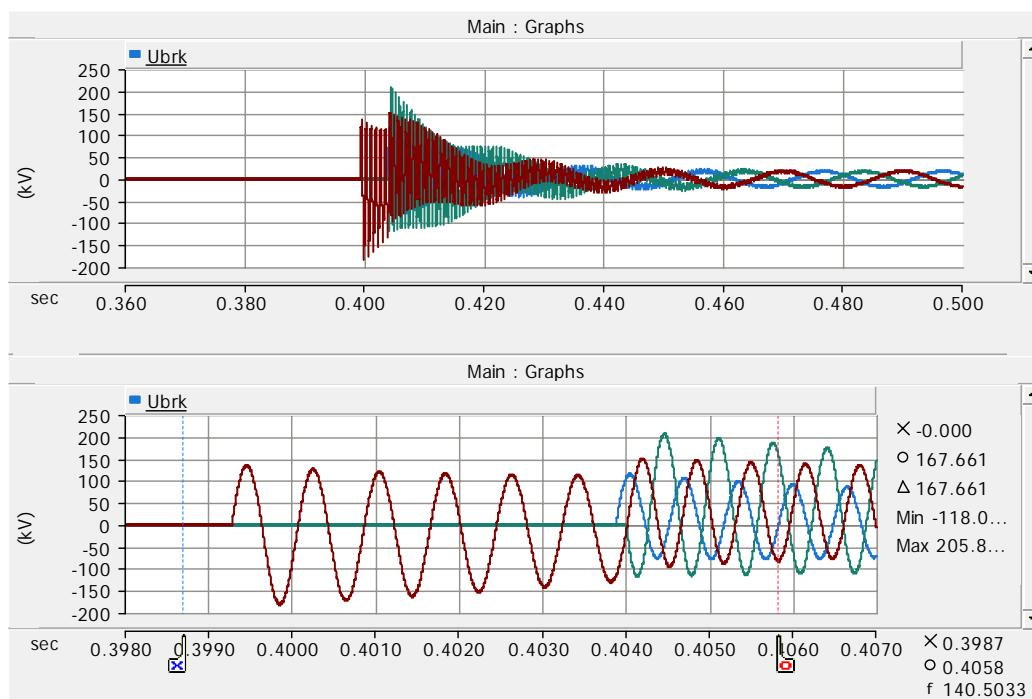
Figure 42. Breaker voltages before cable and reactor on case 20.
