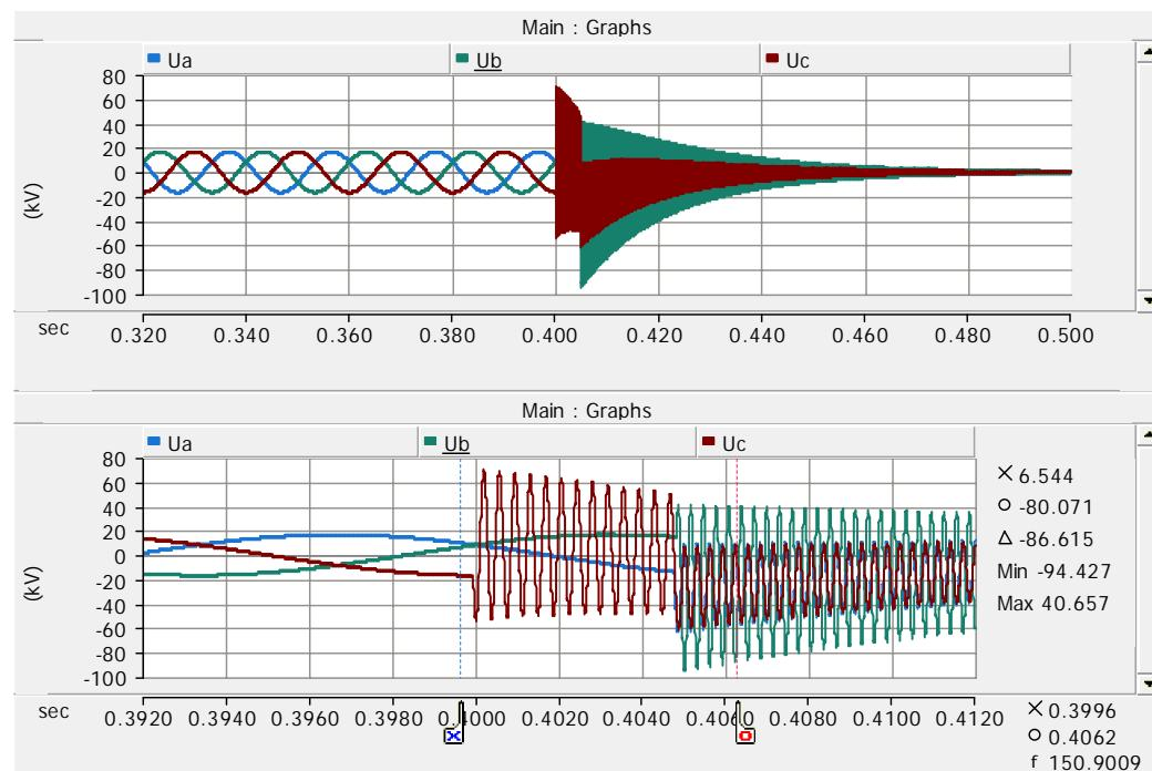
Figure 81. Reactor bus phase voltages on case 88.
