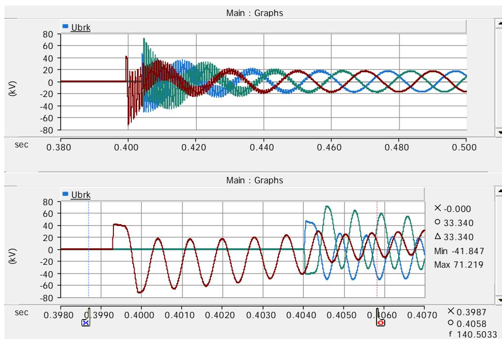
Figure 52. Breaker voltages before cable and reactor on case 32.
