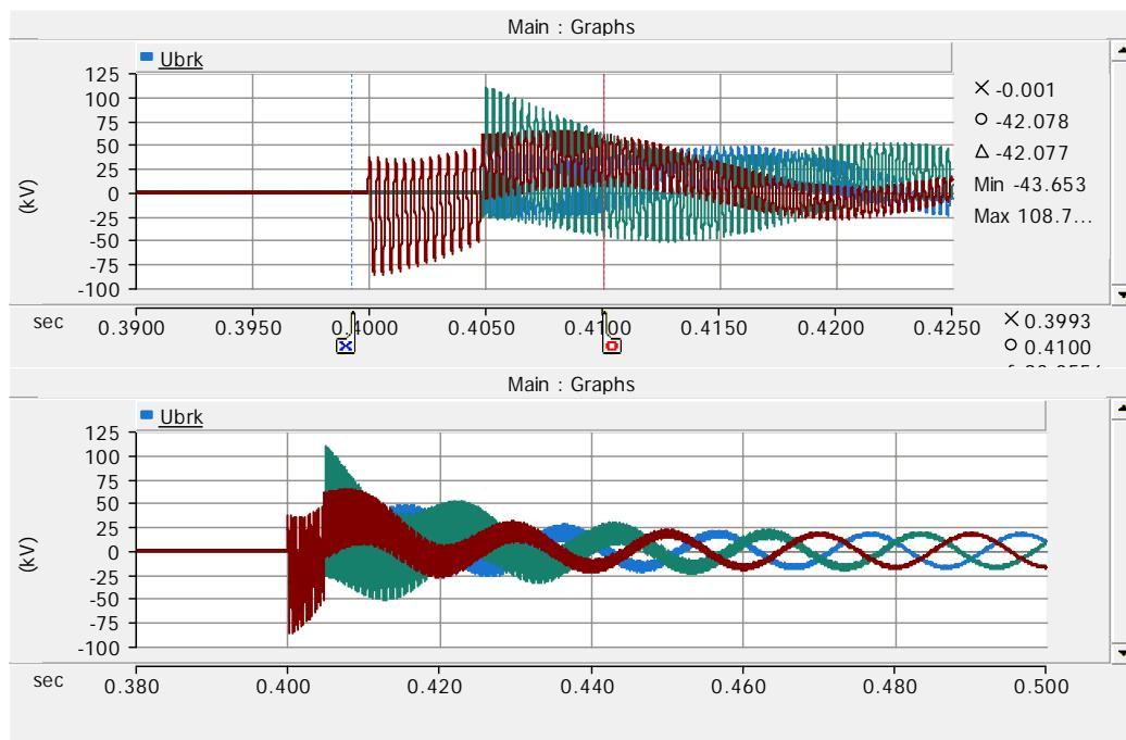
Figure 82. Breaker voltages before cable and reactor on case 88.
