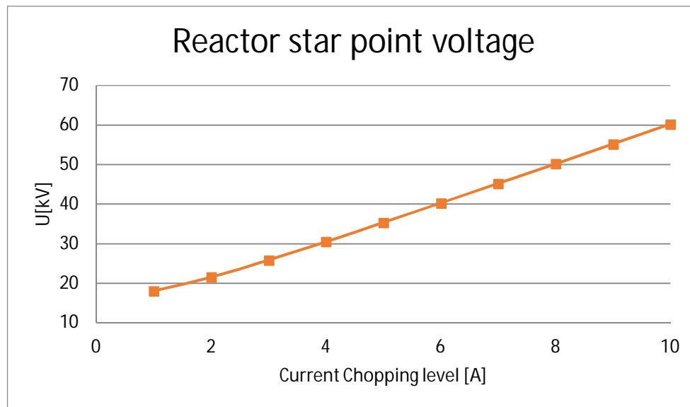
Figure 21. Peak values of shunt reactor star point voltage on cases 11-20 (Reactor 1 MVar, connection cable 50 m, main transformer 25 MVA)
