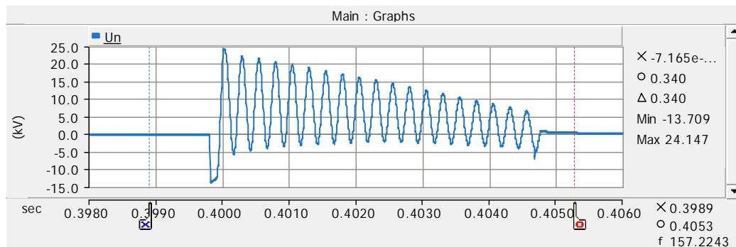
Figure 68. Reactor star point voltage on case 59.
