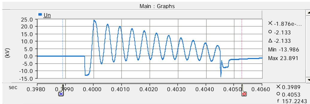
Figure 98. Reactor star point voltage on case 107.
