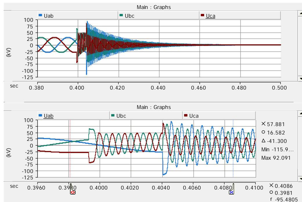
Figure 50. Reactor bus phase to phase voltages on case 32.
