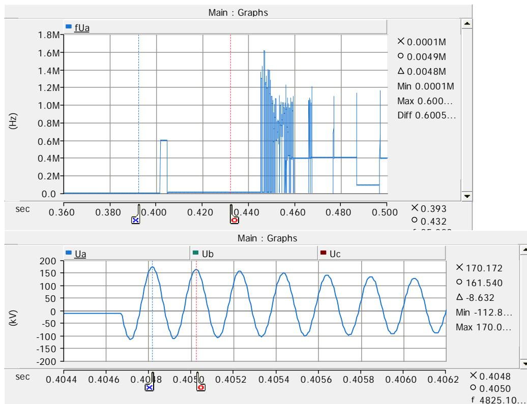
Figure 59.  $U_a$  phase Frequency on case 44.
