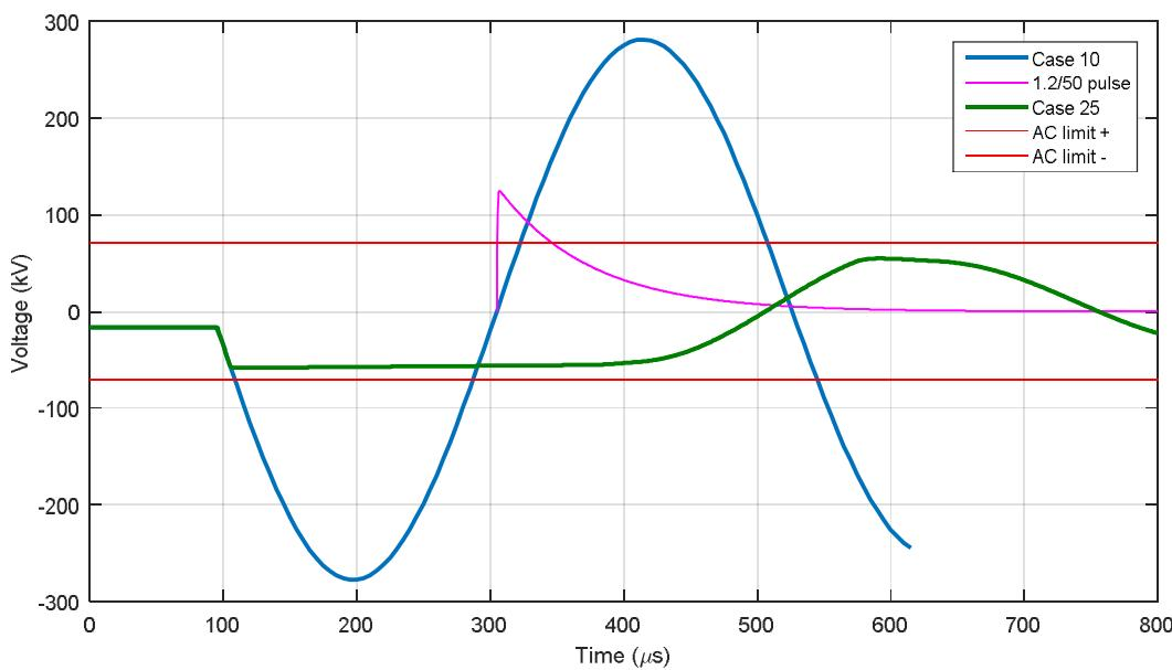
Figure 34. Examples of voltage waveforms in comparison with standard test limits.
