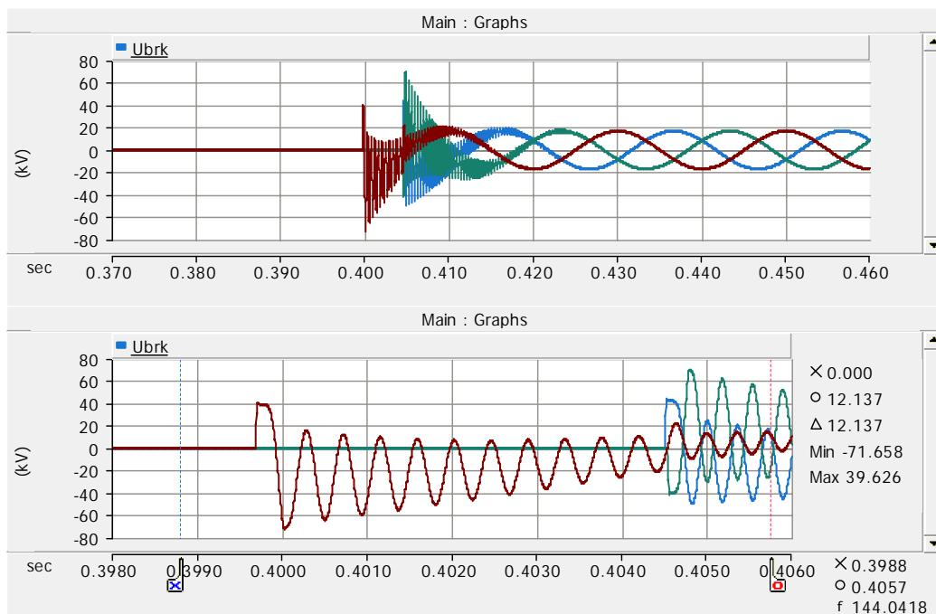
Figure 97. Breaker voltages before cable and reactor on case 107.
