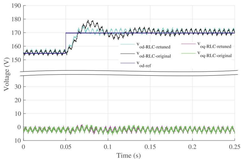
Figure 9. Step response of the grid-forming inverter with problematic RLC-resonant load with original control design (dark blue line) and with specifically tuned control system (light blue).
