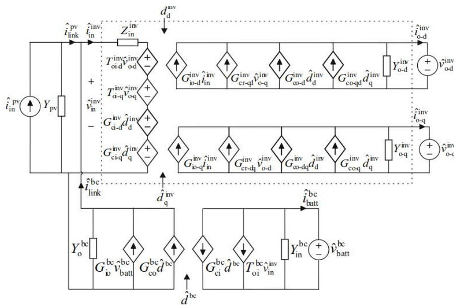
Figure 11. Overview of the complete PV inverter dynamic model with battery storage and DC-DC interfacing converter.
