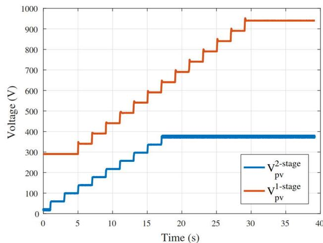
Figure 6. Operating range of the PV generator in single stage topology in red and double stage topology in blue.
