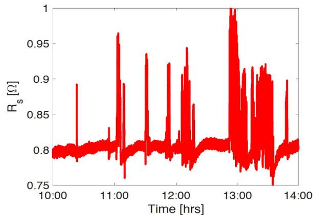
Fig. 15. Identified series resistance from the one-day I-U curve measurements of a PV panel.
