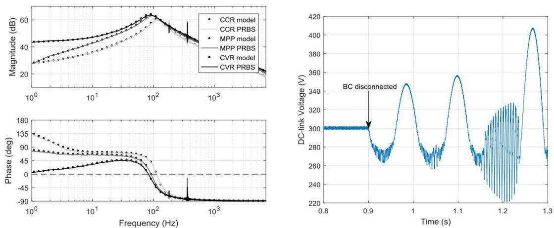
Figure 12. a) Dynamic model of the grid-connected PV inverter with battery storage, represented as a frequency response. b) DC-link voltage of the PV inverter begins oscillating due to unstable control system.
