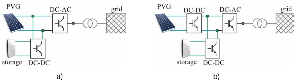
Figure 5. a) Single and b) double stage topologies for PV interfacing energy storage.
