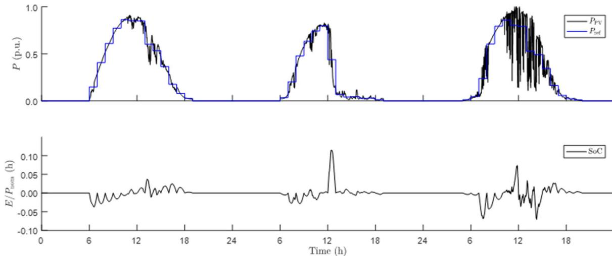
Figure 2. On top is the PV generator output power and the power fed to the grid, i.e., the reference power for state of charge, and down below is the state of charge of ESS during three days from April 11 to 13<sup>th</sup> in 2015.
