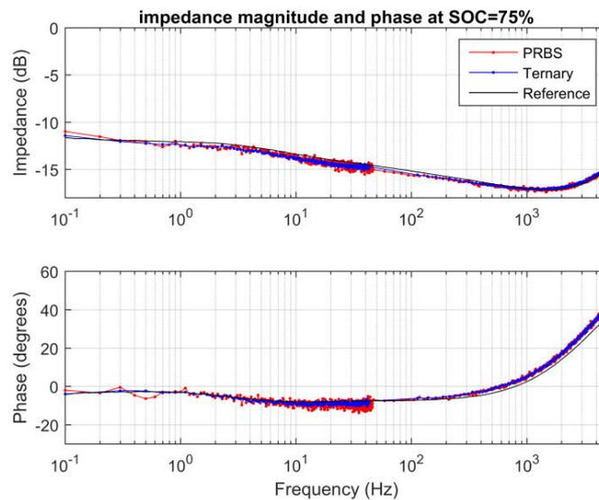
Figure 10. Measured internal impedance of a Li-ion battery pack using the conventional sine-sweep method (in blue) and the PRBS-method (in red).
