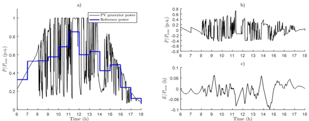
Figure 3. a) 10 MW PV generator power and the grid feeding reference power with 60 min ISP, b) the corresponding power taken from the ESS and c) the energy stored in ESS (state of charge) on 17<sup>th</sup> of June 2015.
