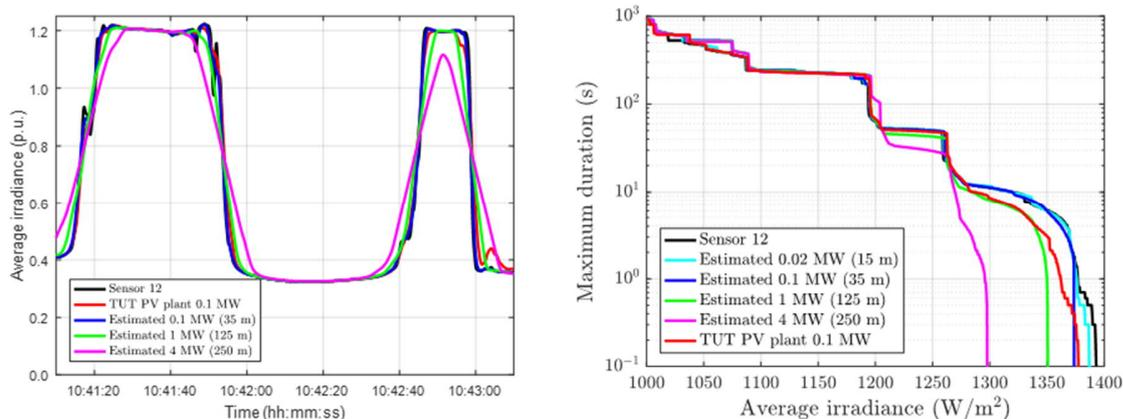
Figure 4. On the left is an example of cloud enhancement effect on different PV generator sizes. On the right is the maximum duration of the enhanced irradiance over different PV generator sizes during 23 summer months from 2014 to 2018.
