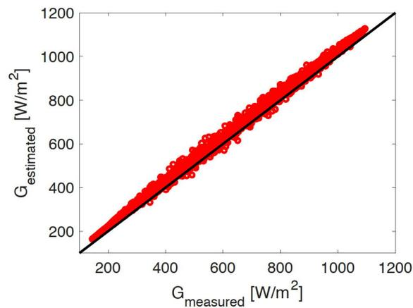
Fig. 14. Scatter plot of the estimated vs. measured irradiances during one-day I-U curve measurements of a PV panel.
