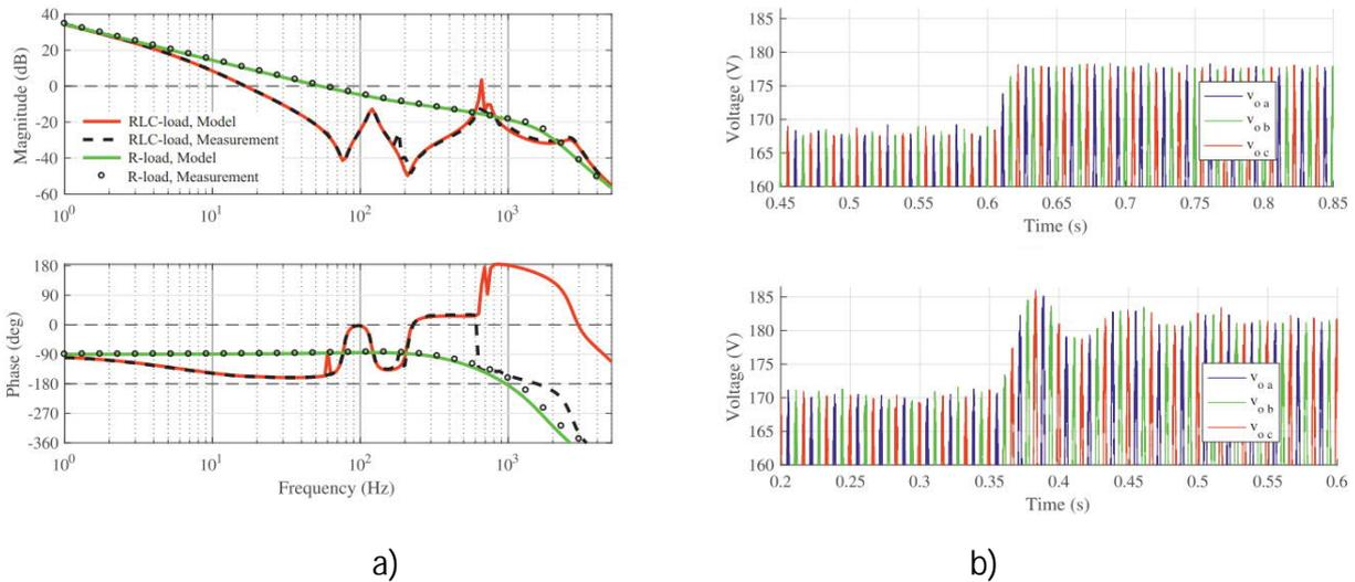
Figure 8. a) Control loop gains of the grid-forming inverter obtained from the developed dynamic model with two different load impedances. b) Time-domain responses after sudden load changes.
