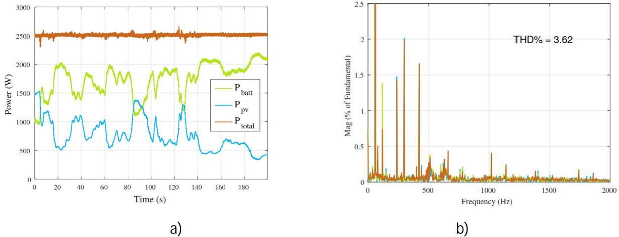
Figure 7. a) Power generated by the PV, absorbed by the battery and fed to the grid. b) Total harmonic distortion of grid currents.
