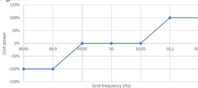
Figure 4 Operation of a reserve unit in primary frequency regulation according to minimum frequency requirements by Fingrid [8] [9]
