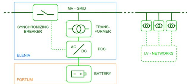
Figure 1, Conceptual drawing of the battery system and ownership lines
